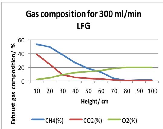
Figure 2c Black soil with 300 ml/min of LFG
