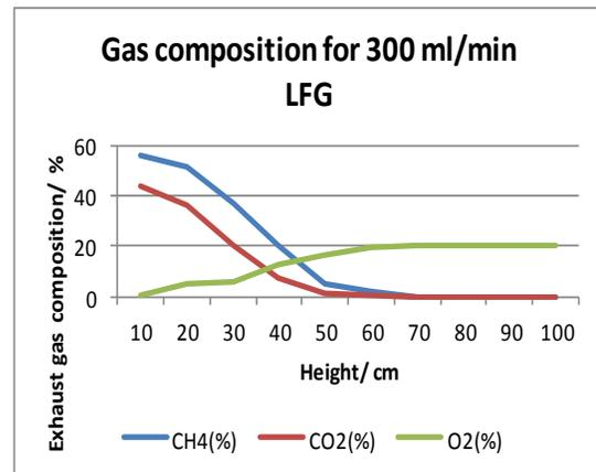
Figure 3c Compost with 300 ml/min of LFG
