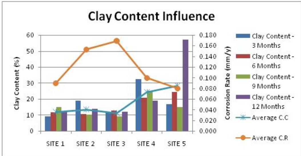
Figure 8: Relationship between corrosion rate and clay content
