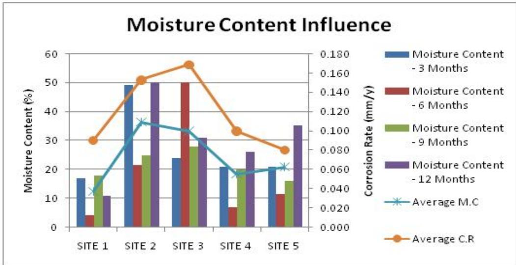
Figure 7: Relationship between corrosion rate and moisture content
