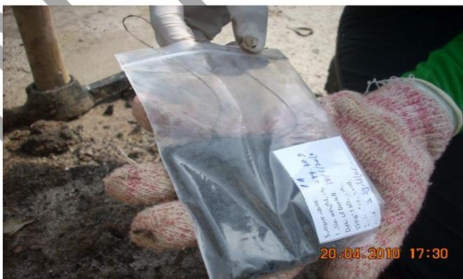
Figure 4: Retrieved sample in a sealed plastic bag
