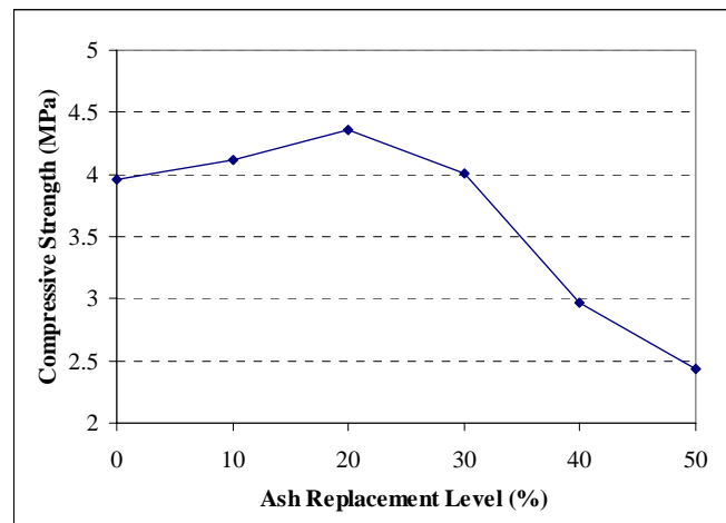
Figure 3 : Effect of POFA content on compressive strength of aerated concrete
