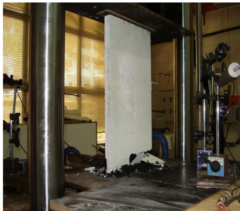
Figure 11: Crushing failure at lower part
