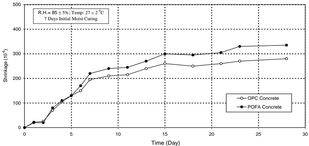
Figure 3: Shrinkage of OPC concrete and POFA concrete
