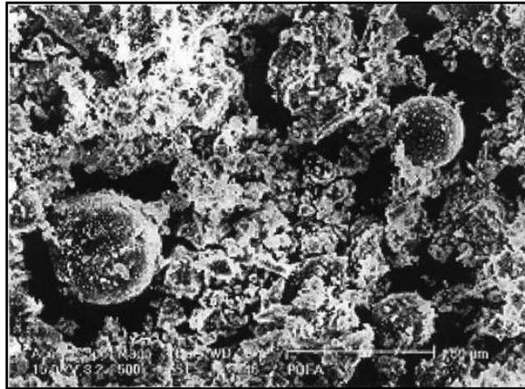
Figure 2: Scanning electron micrograph of POFA
