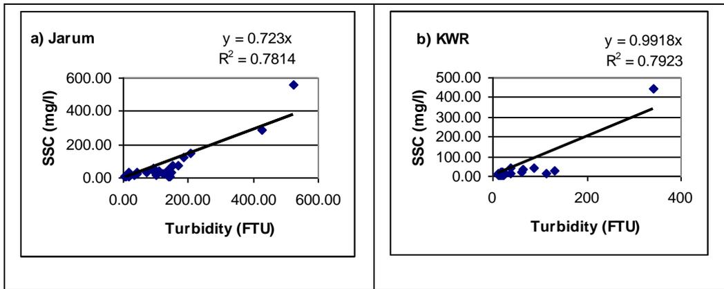
Figure 3 : The relationship between SSC and turbidity at (a) Jarum river (R1) and (b) KWR river (R2) based on fortnightly sampling data
