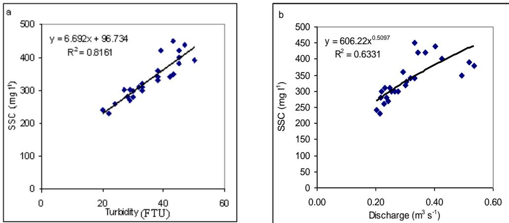
Figure 9 : Relationship between: (a) turbidity and SSC, and (b) discharge and SSC during storm event on 11/10/2001 to 12/10/2001 at R2
