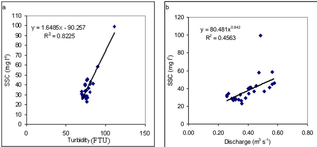
Figure 7 : Relationship between: (a) turbidity and SSC, and (b) discharge and SSC during storm event on 11/10/2001 to 12/10/2001 at R1
