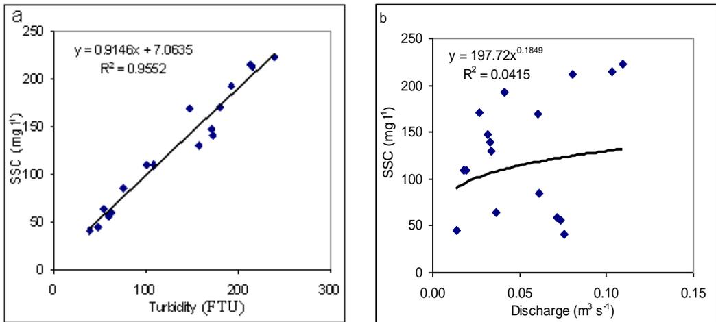
Figure 8 : Relationship between: (a) turbidity and SSC, and (b) discharge and SSC during storm event on 1/10/2001 to 4/10/2001 at R2.
