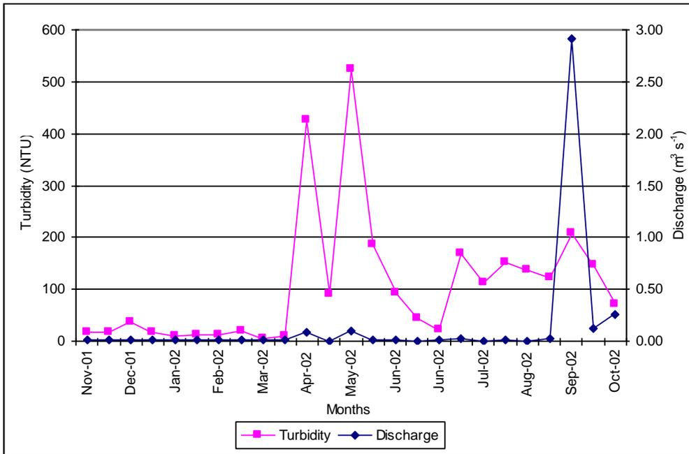
Figure 4 : Relationship between turbidity and discharge at R1
