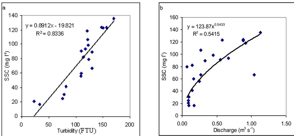
Figure 6 : Relationship between: (a) turbidity and SSC, and (b) discharge and SSC during storm event on 1/10/2001 to 4/10/2001 at R1
