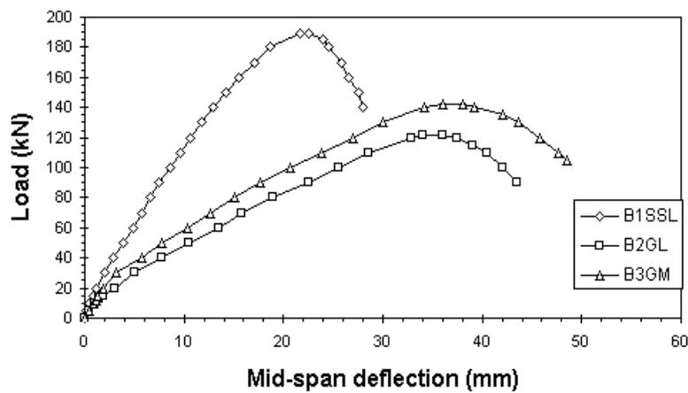
Figure 2: Load-deflection of all beams tested
