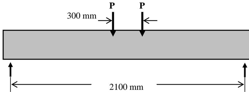
Figure 1: Schematic diagram of the test set-up
