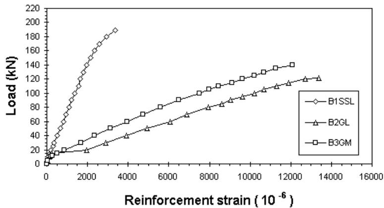
Figure 4: Load-reinforcement strain for all beams tested
