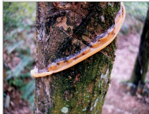
Photo 2: Spirally fitted rubber collar for intercepting stemflow.
