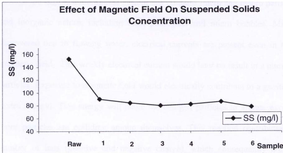
**Figure 5 :** Suspended Solids Concentration After Passing Magnetic Field
