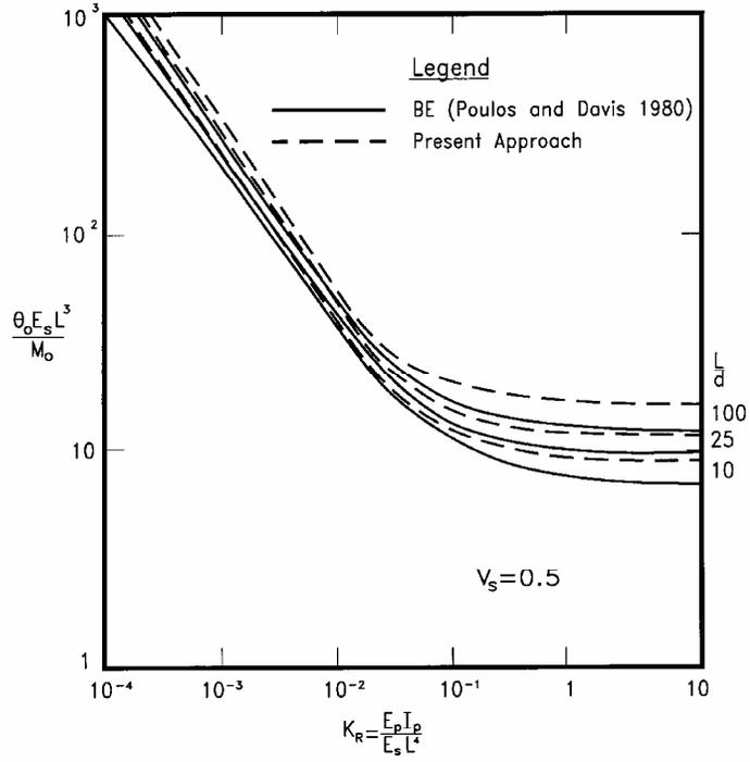
**Figure 4 :** Normalized Head Rotation Response for Free-Head Pile
