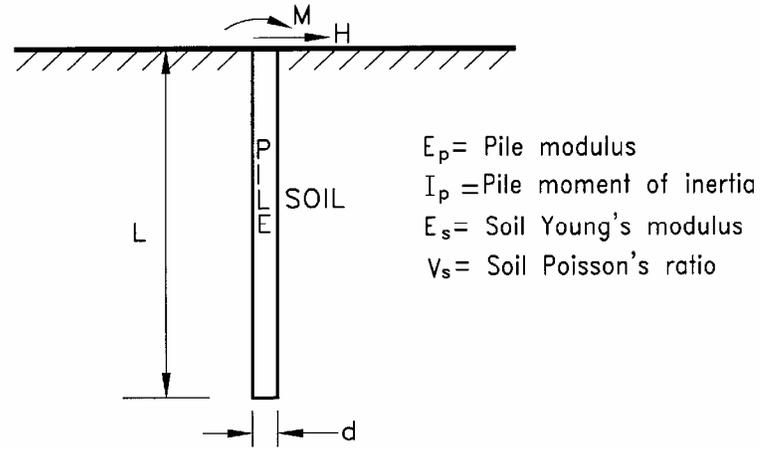
**Figure 1** : Definition of Laterally Loaded Pile Problem
