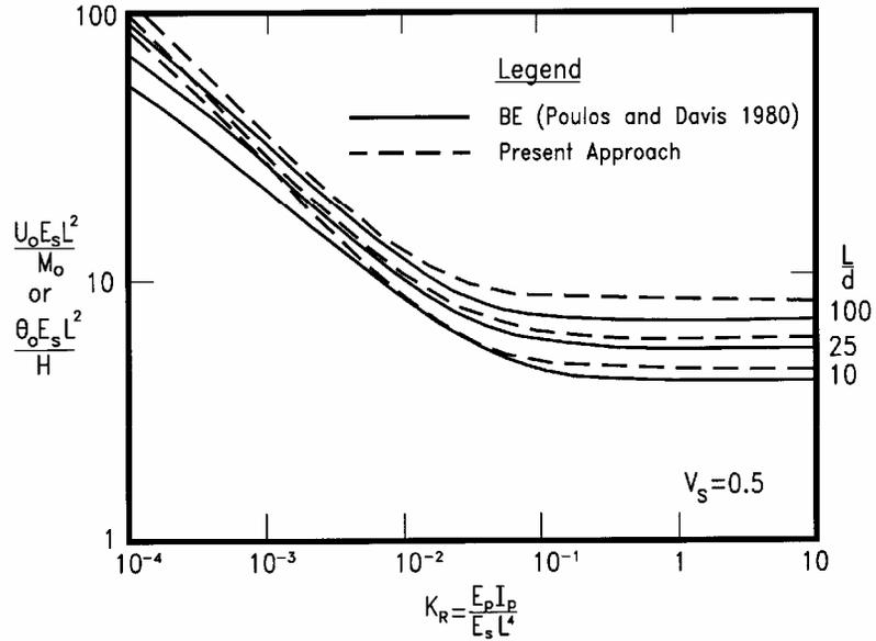
**Figure 3 :** Normalized Head Deflection (or Rotation) Response for Free-Head Pile
