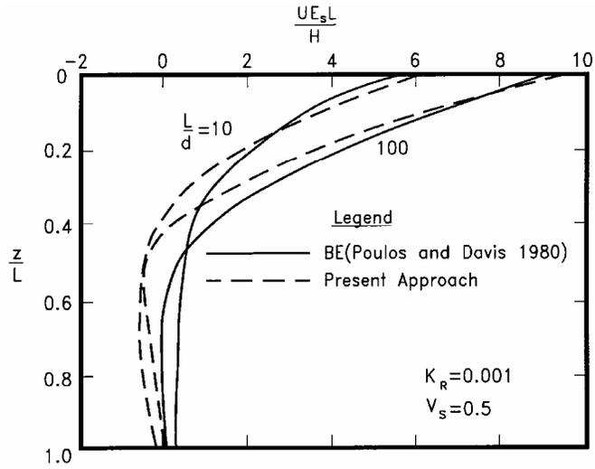
**Figure 5 :** Deflection Profile Along Free-Head Pile
