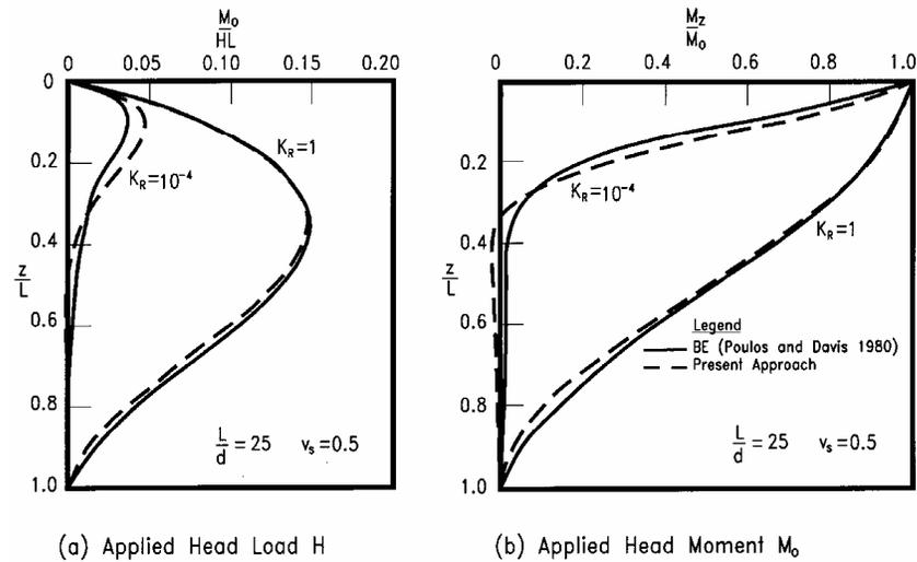
**Figure 6 :** Moment Profile Along Free-Head Pile
