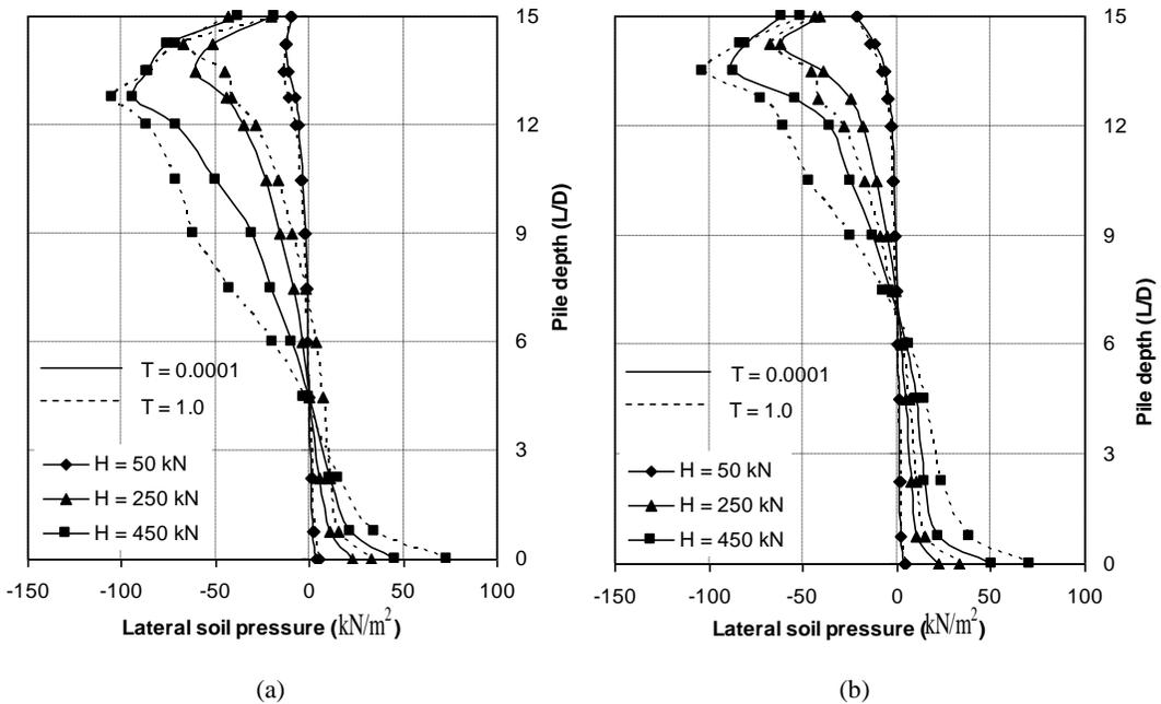
Fig 10. Lateral soil resistance with depth, (a) cohesionless soil, (b) cohesive soil
