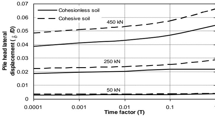
Figure 7. The predicted pile head lateral displacement with time based on three lateral loads intensities
