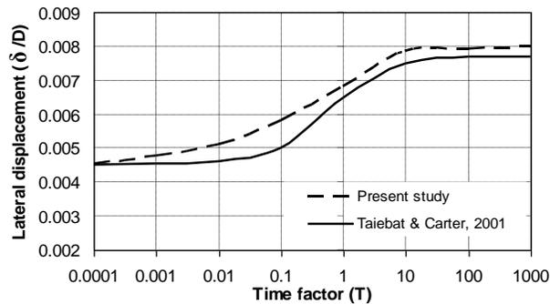
Figure 4: Comparison of the lateral displacements of the pile head in elasto-plastic soils.
