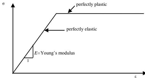
Figure 1: Stress – strain curve (Johnson et al., 2006)
