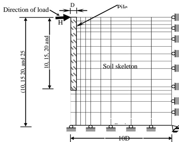
Fig. 3: 2-Dimensional finite element mesh.
