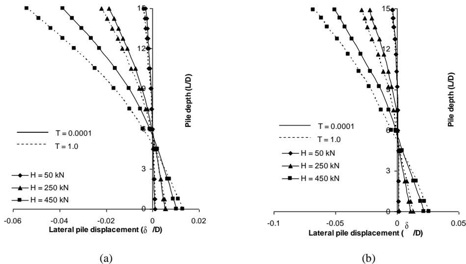
Figure 6. Lateral pile displacement with depth, (a) cohesionless soil, (b) cohesive soil
