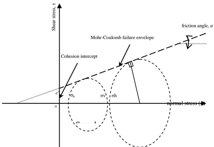
Figure 2: Mohr-Coulomb's failure surface (Potts & Zdravkovic, 1999)
