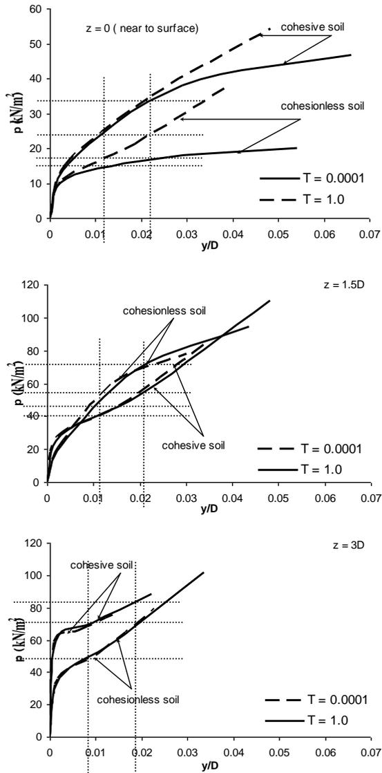
Figure 11.  $p$ - $y$  curves predicted from the finite element simulation under the effect of time-dependent and with different depth below pile tip of pile embedded on two types of soil,  $L = 15\text{m}$
