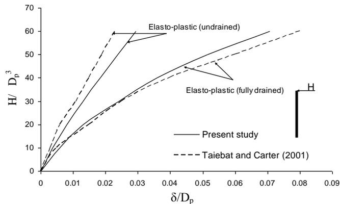
Figure 5: Lateral displacement relationships for laterally loaded piles under drained and undrained conditions
