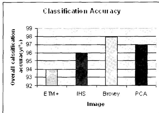
Figure 3.1 : Resulting overall classification accuracy of supervised maximum likelihood classification using ETM+ and fused images of IHS, Brovey and PCA
