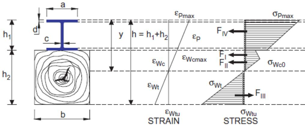
Figure 10 : Cross-section stress and strain analysis
