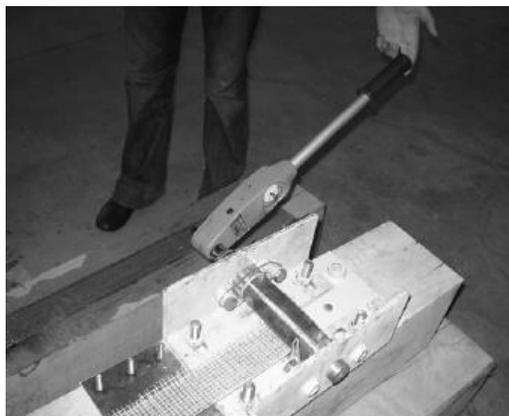
Figure 13 : Fixing the strips using the metal cylinder
