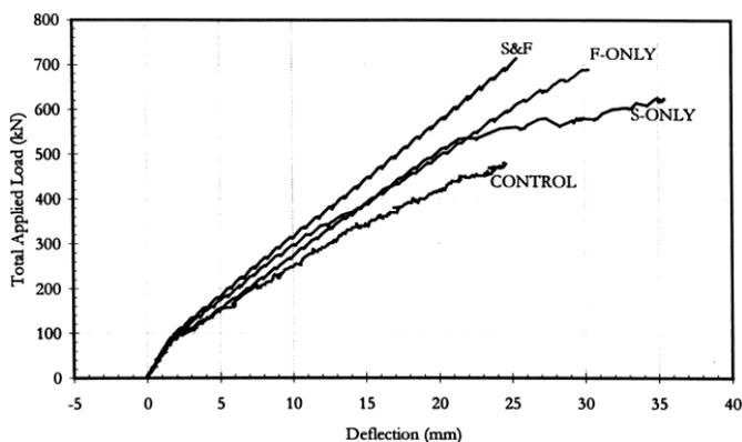
Figure 2: Behavior of strengthened and control beams
