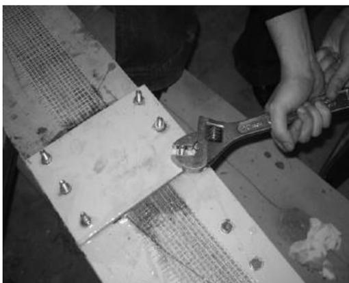
Figure 14 : Fixing the strips using the clamp
