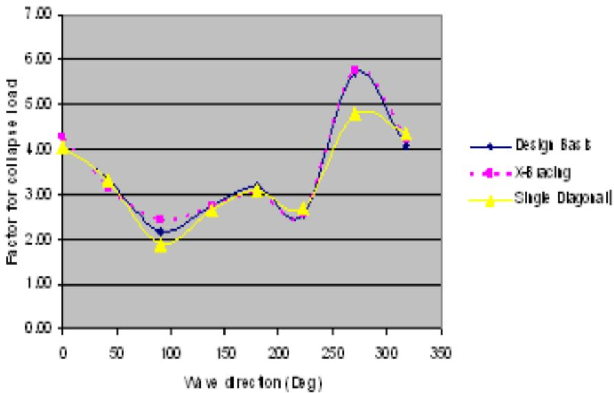
Figure 14: Collapse Load factor Vs Wave direction
