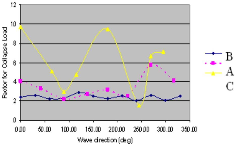
Figure 8: Collapse Load factor VS Wave Direction
