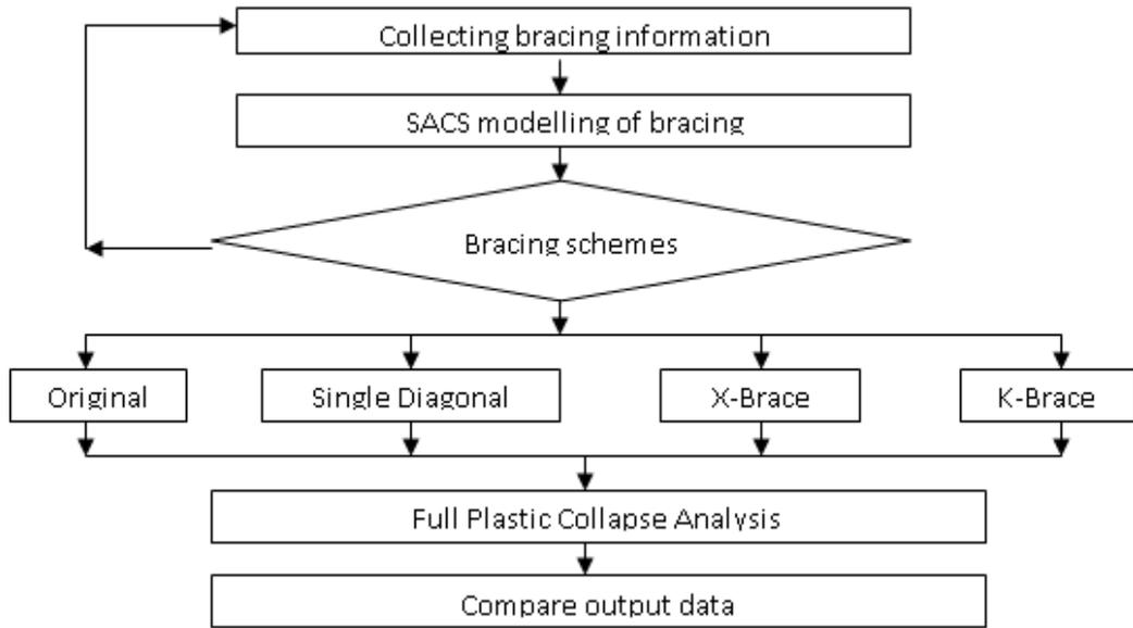
Figure 3: Flow chart of bracing configuration study (Fawaz, 2010)
