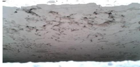
Figure 8: Porous Defect
