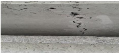
Figure 4: Tearing defect
