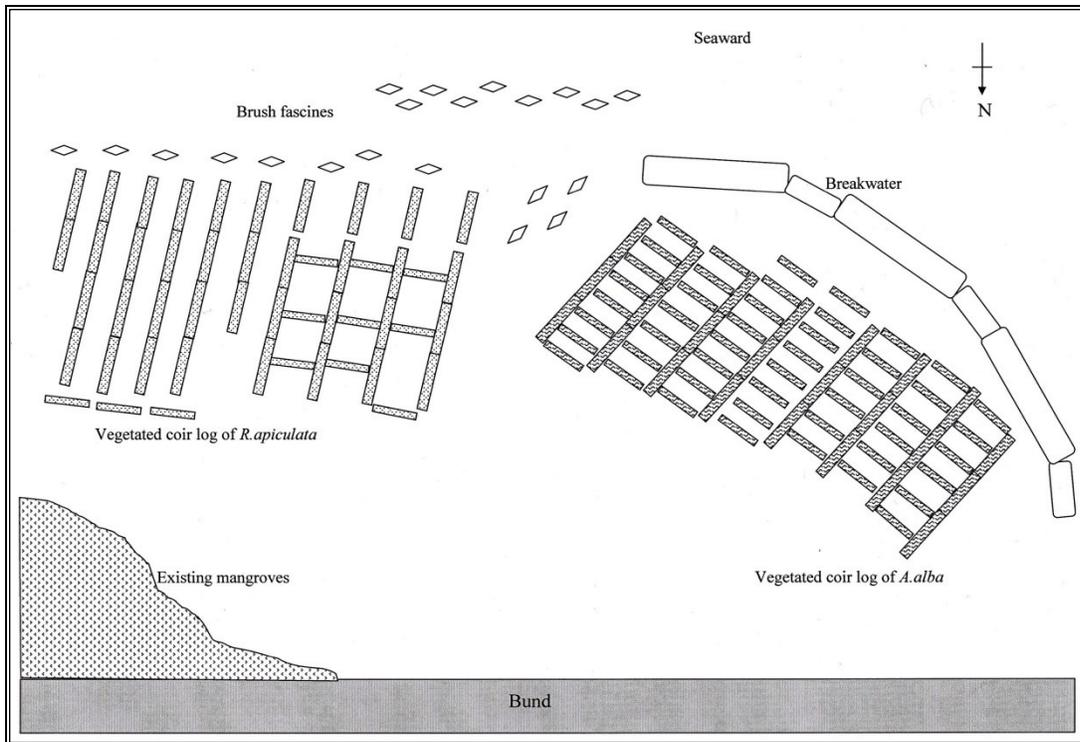
Figure 2. Formation of vegetated coir logs arranged in grid planted behind the breakwater.
