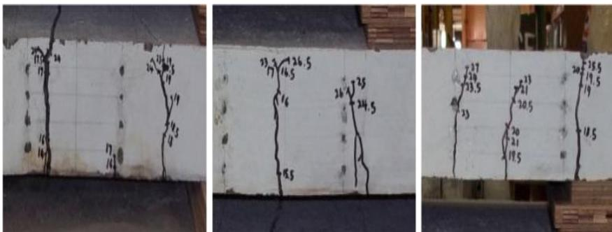
Figure 11: Cracking pattern of concrete slabs (from left to right: NC, SCC, 1.0%GFRSCC)
