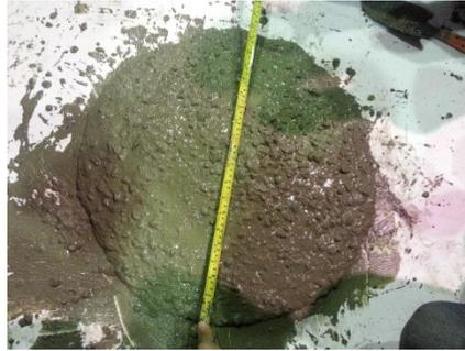
Figure 1: Slump flow test
