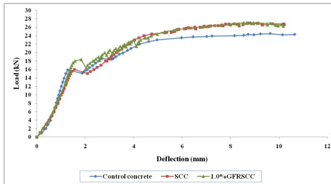
Figure 10: Load deflection curves for control concrete, plain SCC, and 1.0% GFRSCC slabs
