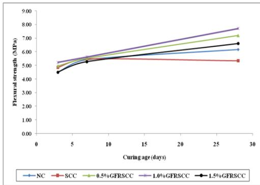
Figure 8: Relation between flexural strength and curing age
