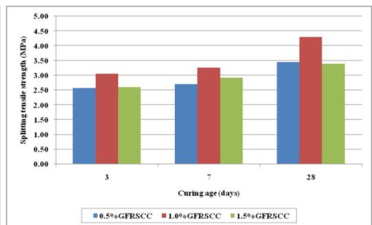
Figure 7: Splitting tensile strength of GFRSCC samples
