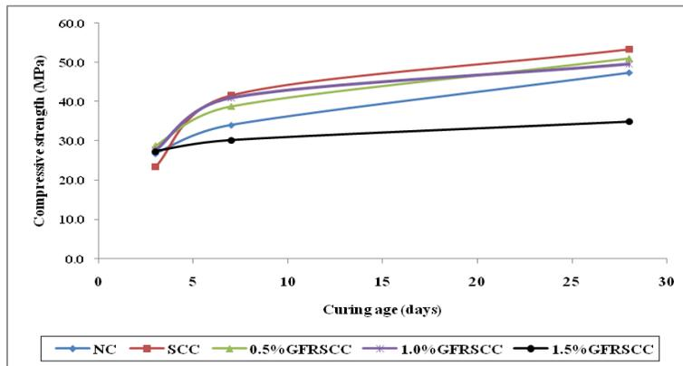
Figure 5: Relation between compressive strength and curing age for each type of concretes
