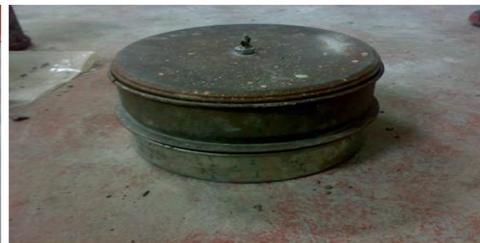
Figure 3: Sieve for segregation resistance test
