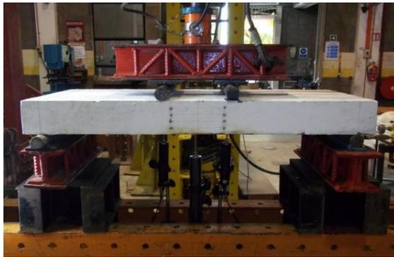
Figure 4: Setup of small-scale slab test
