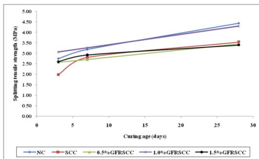
Figure 6: Relation between splitting tensile and curing age
