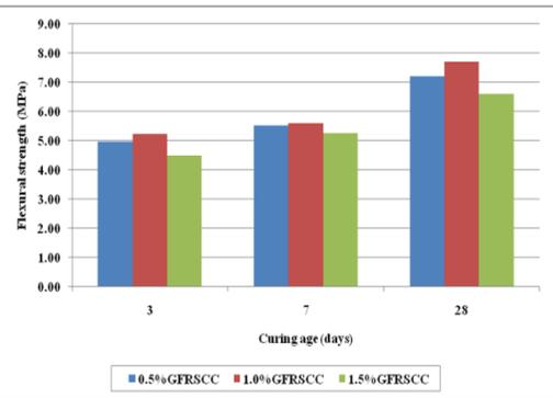
Figure 9: Flexural strength of GFRSCC samples
