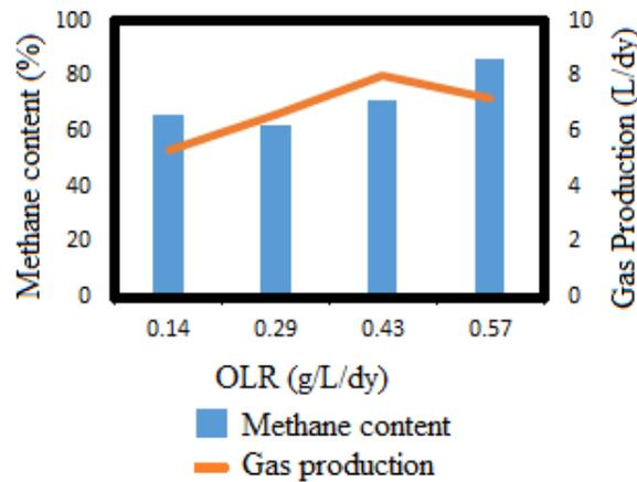
**Figure 5:** Variation of biogas against various loading rates
