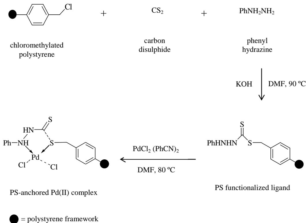
Scheme 1: Synthesis of the PS-anchored Pd(II) complex
