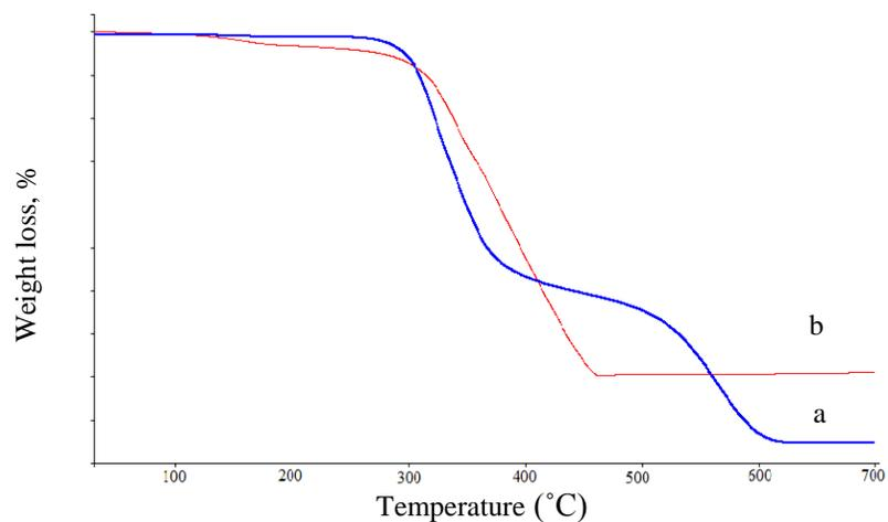
Figure 3: TGA curves for the (a) parent PS (b) PS-anchored Pd(II) complex
