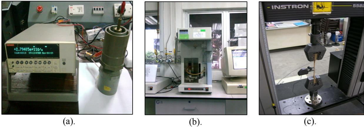
Figure 2: (a) Electrical resistivity, (b) thermal stability, and (c) tensile strength test set-up.
