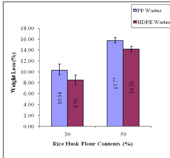
Figure 6: Mean weight loss (WL) value of RPC made from different plastic waste materials and RHF contents.
