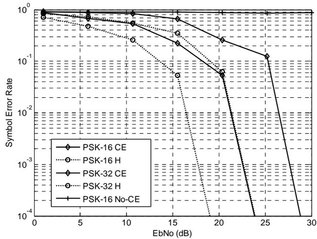
Figure 5 : Performance comparison of least square error estimation with different modulation techniques
