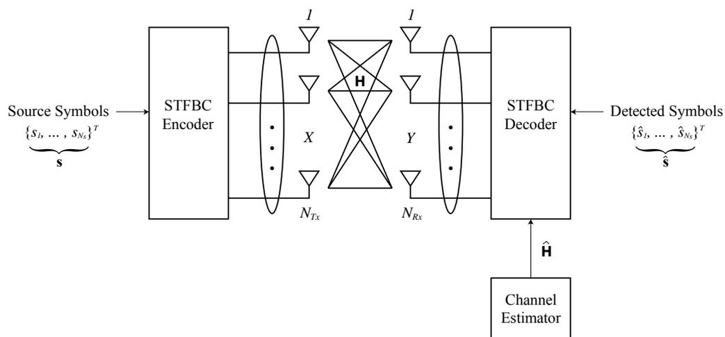
Figure 1 : Block diagram of STFBC
