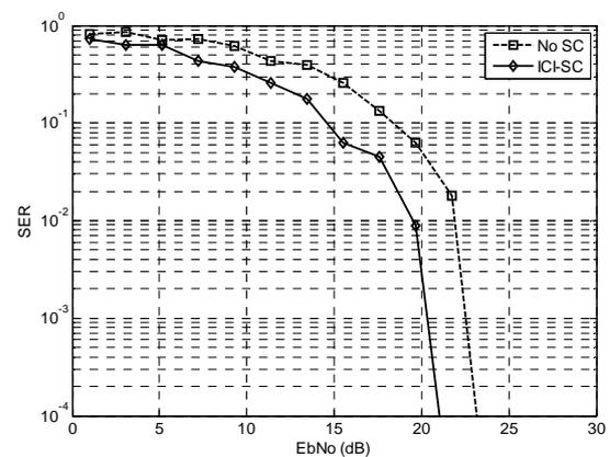
Figure 4 : Performance improvement with and without ICI-SC using median method
