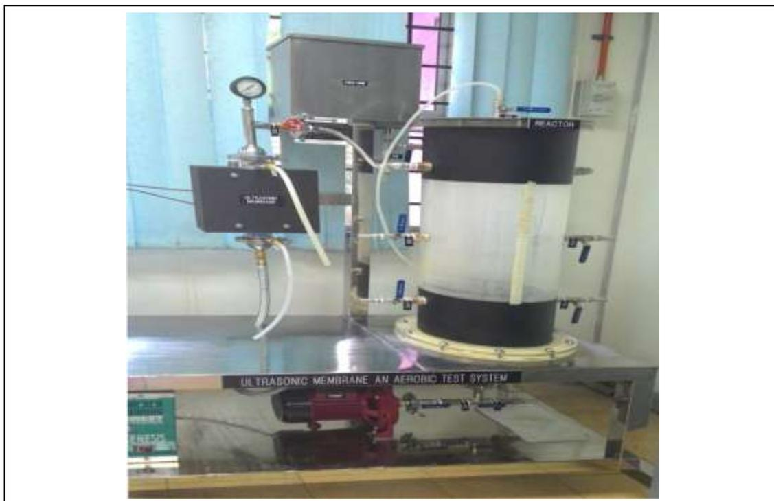
Fig. 2. Membrane Anaerobic Reactor (MAS) System in Environmental Laboratory
