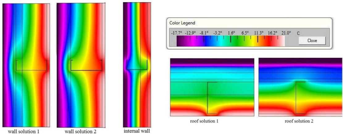
Figure 2: Temperature variation through wall and roof from Therm-5
