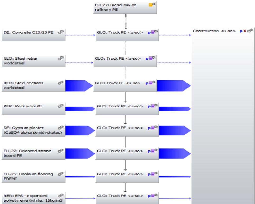
Figure 4: Construction phase with transportation in software GaBi.
