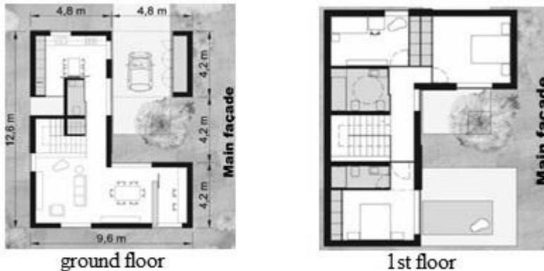
Figure 1: Ground floor and 1<sup>st</sup> floor plan
