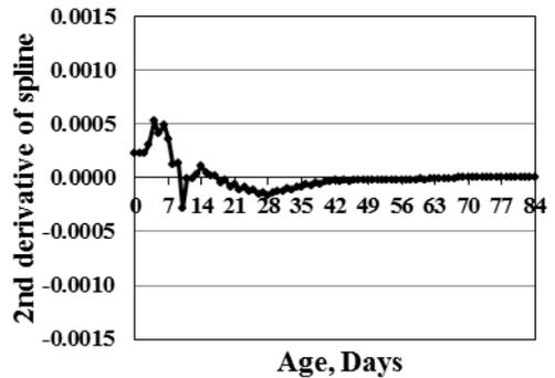
Figure 4: 2<sup>nd</sup> Derivative of Spline Curve for Reactive Aggregate-I Expansion
