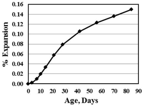
Figure 1: Experimental Percent Expansion Curve for Reactive Aggregate-I
