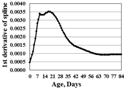
Figure 3: 1<sup>st</sup> Derivative (slope) of Spline Curve for Reactive Aggregate-I Expansion
