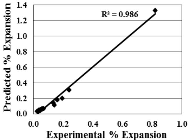
Figure 8: Combined Comparison of % Expansion for Aggregates and Aggregates with Mitigation
