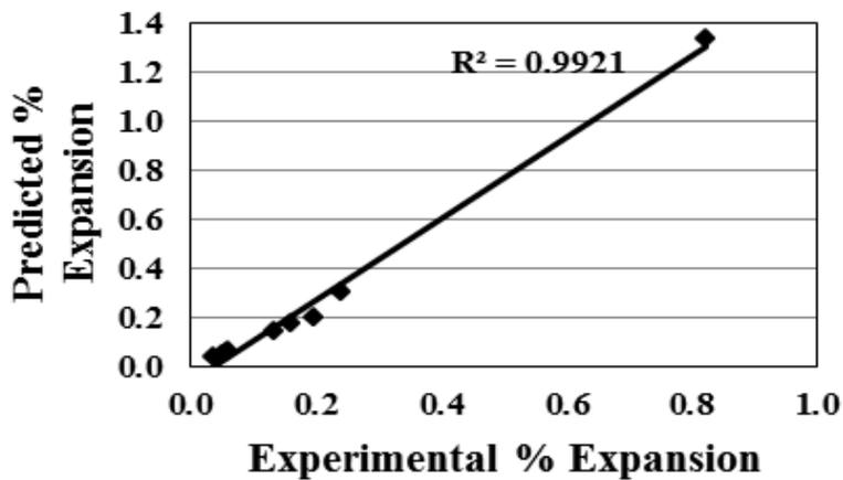
Figure 6: Comparison of Percent Expansion for reactive and non-reactive Aggregates
