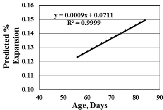
Figure 5: Predicted Percent Expansion Curve for Reactive Aggregate-I (56 to 84 Days)
