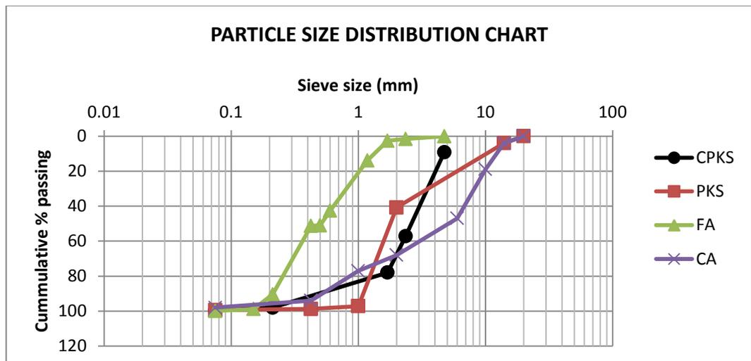
Figure 3: Particle Distribution Curves for Crushed Palm Kernel Shell, Palm Kernel Shell, Fine Aggregate and Coarse Aggregate.
