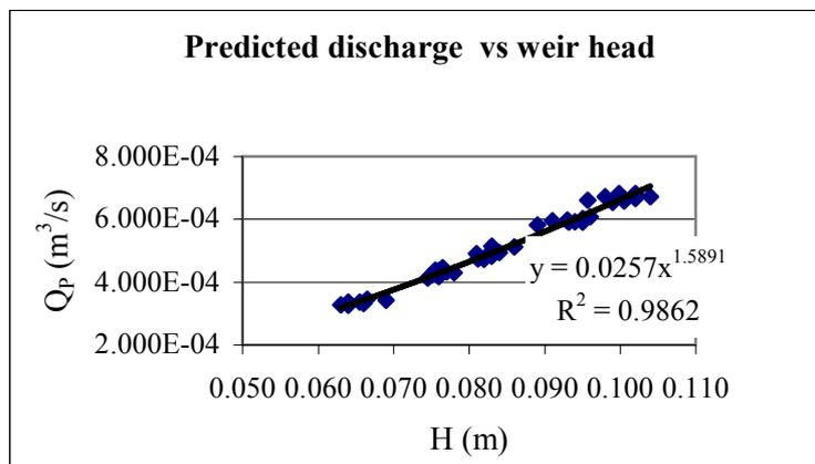
Figure 4: Predicted discharge  $Q_P$  plotted against weir head  $H$  for head-discharge relationship of contracted rectangular flat-crested slit weir
