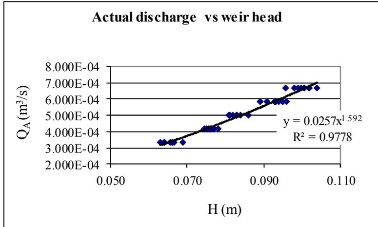
Figure 3: Actual discharge  $Q_A$  plotted against weir head  $H$  for head-discharge relationship of contracted rectangular flat-crested slit weir
