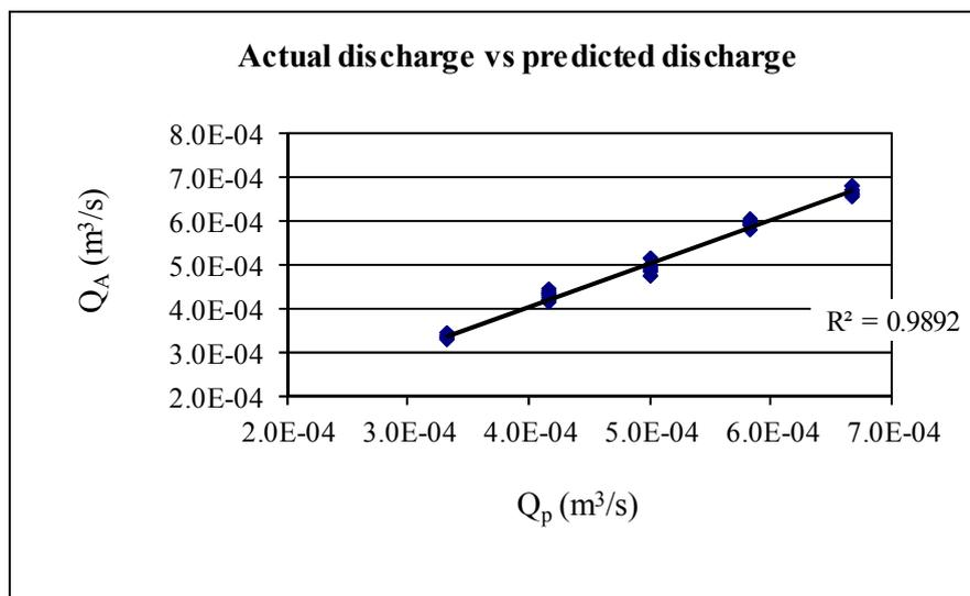
**Figure 5:** Actual discharge  $Q_A$  plotted against predicted discharge  $Q_P$  for contracted rectangular flat-crested slit weir
