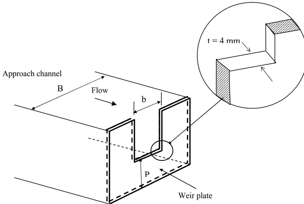
Figure 2: Sketch of contracted rectangular flat-crested slit weir
