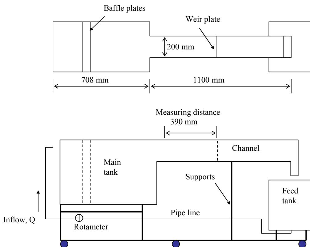
Figure 1: Top and side views of the experimental apparatus
