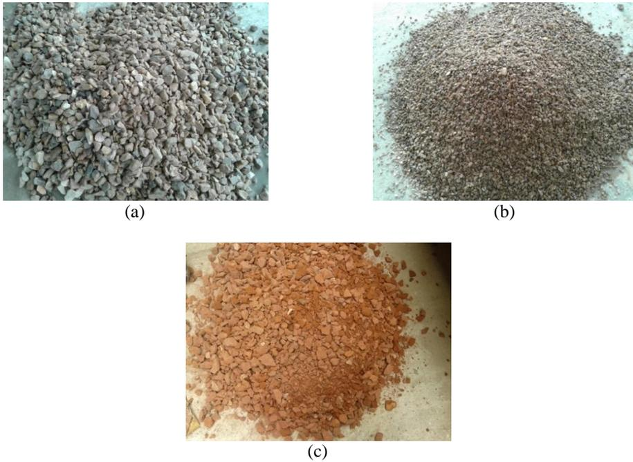
Figure1: (a) 3/4 inch downgraded crushed stone (SC) (b) 3/8 inch downgraded crushed stone (SC) (c) 3/4 inch and 3/8 inch downgraded crushed brick mixed together (BC)
