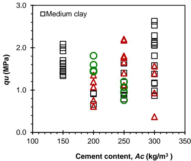
Figure 11: Soilcrete strength,  $q_u$  versus soil types
