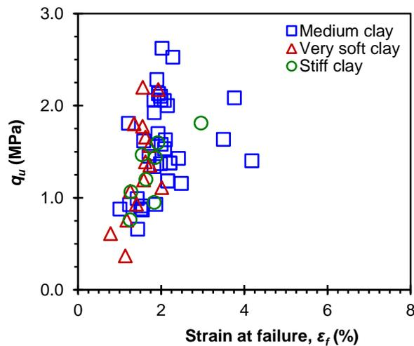
Figure 13: Strain at failure of soilcrete specimens,  $\epsilon_f$
