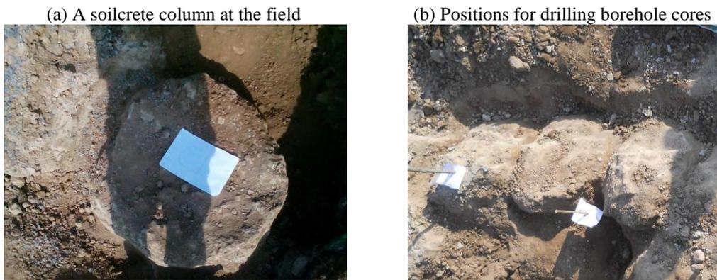
Figure 5: Demonstration of excavation to expose soilcrete columns at the field
