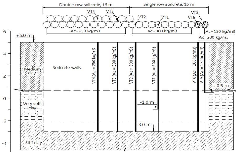
Figure 9: Locations of the drilling core boreholes to take field soilcrete samples and appearance of soilcrete along the soilcrete columns
