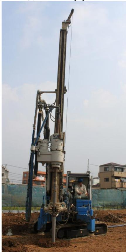
Figure 4: The NSV equipment used for the field construction in Dong Thap province, Vietnam
