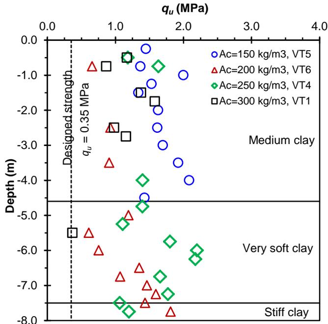
Figure 12: Soilcrete strength,  $q_u$  varying with cement contents and depth
