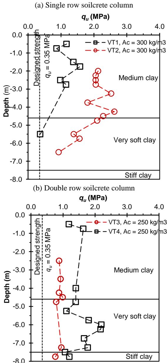
Figure 10: Unconfined compressive strength versus soilcrete depth
