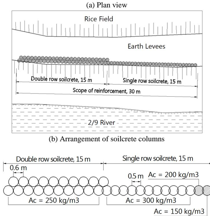
Figure 2: A 30-m trial reinforcement using the NSV system in Dong Thap province, Vietnam
