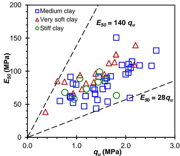
Figure 14: Secant modulus of elasticity,  $E_{50}$  versus  $q_u$
