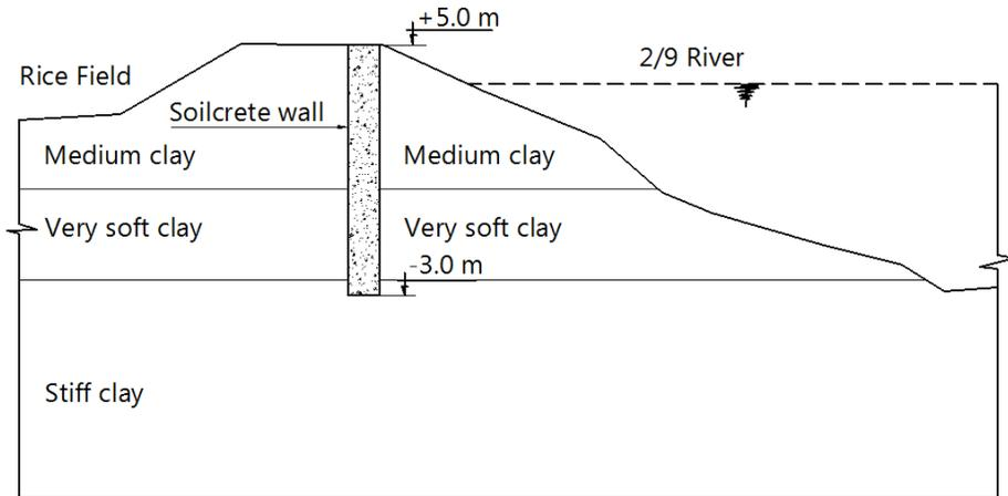
Figure 3: A typical cross-section of the reinforced earth levee in Dong Thap province, Vietnam
