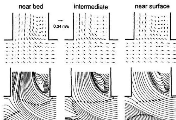
Figure 5: Streamline patterns in smooth branching channel junction bed (Neary & Odgaard, 1993).
