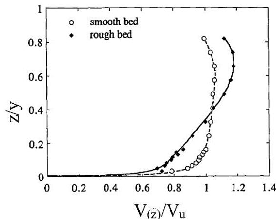
Figure 7: Velocity profiles in main channel (Neary & Odgaard, 1993)
