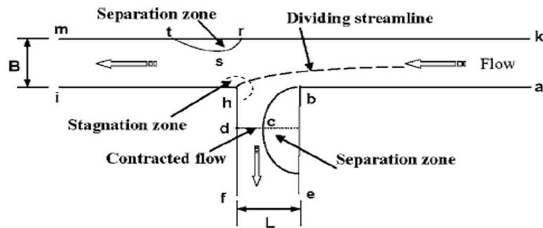
Figure 6: Zones of separation and stagnation point in the branching channel system (Ramamurthy et al., 2007).
