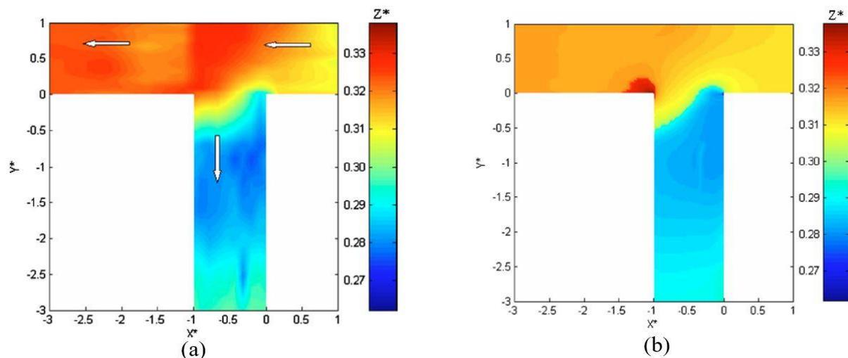
*Figure 3: Water surface profiles for  $Q_r = 83.8\%$ . (a) Experimental data, (b) Numerical model (Ramamurthy et al., 2007).*
