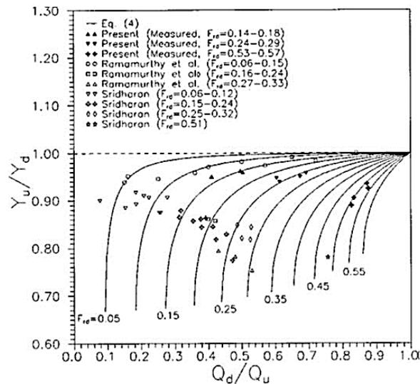
Figure 4: The relationship between  $(y_u/y_d)$ ,  $(F_d)$ , and  $(Q_d/Q_u)$  (Hsu et al., 2002).
