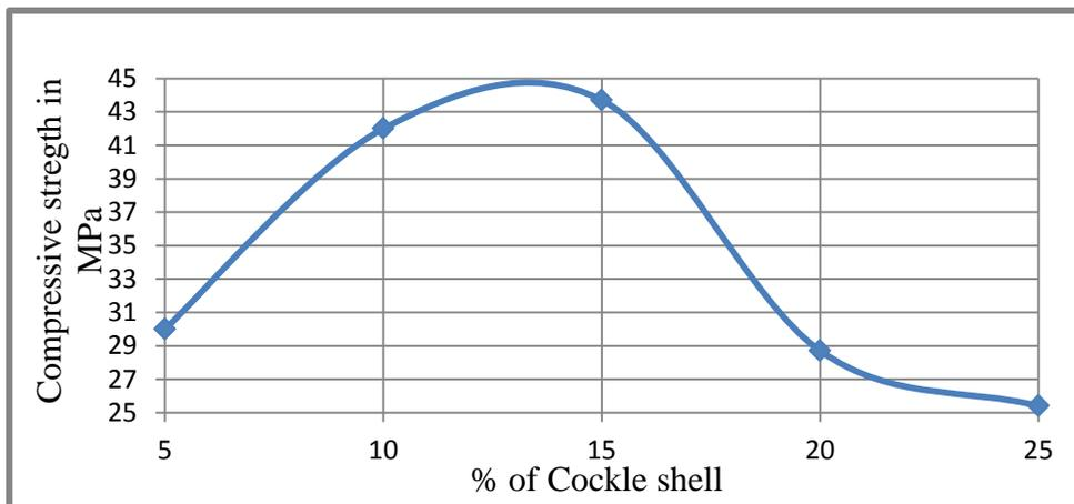
Figure 9 (a): Compressive strength of concrete with different percentage of cockle shell (granite powder 20% fixed)
