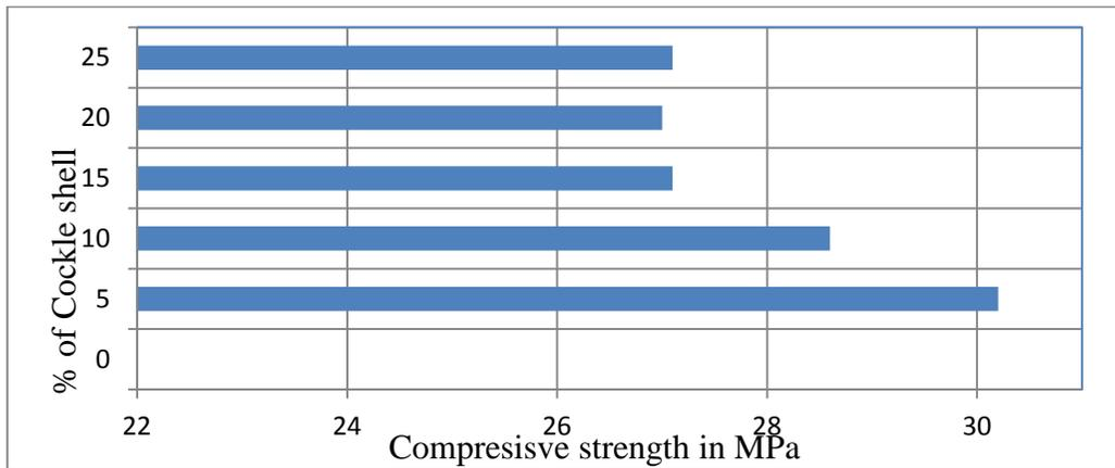
Figure 10 (b): Compressive strength of concrete at different percentage of cockle shell (granite powder 25% fixed)
