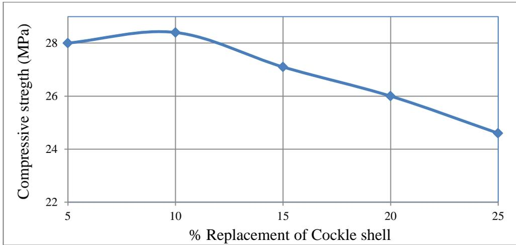
Figure 5 (a): Compressive strength of concrete at different percentage of cockle shell
