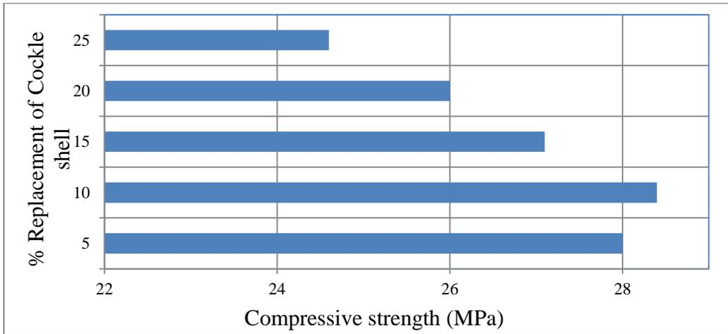
Figure 5 (b): Compressive strength of concrete at different percentage of cockle shell
