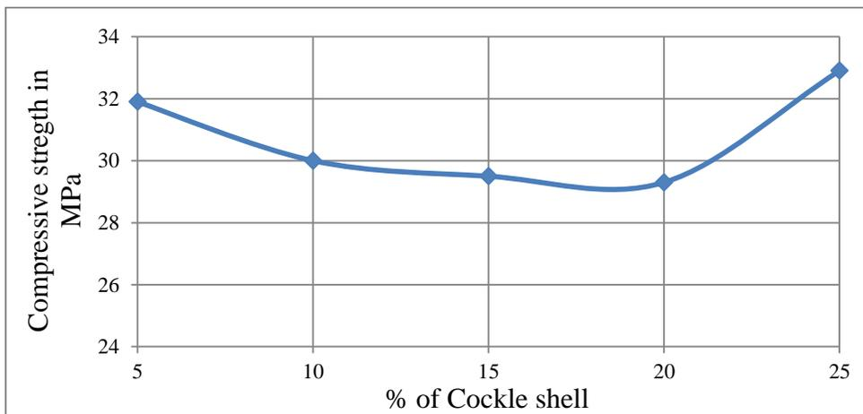
Figure 8 (a): Compressive Strength of concrete with different percentage of cockle shell (granite powder 15% fixed)
