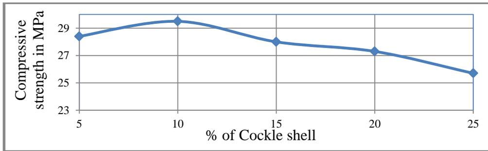
Figure 6 (a): Compressive strength of concrete with different percentage of cockle shell (granite powder 5% fixed)
