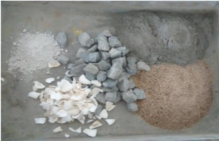
Figure 3: Ingredients of concrete including cockle shell and granite powder
