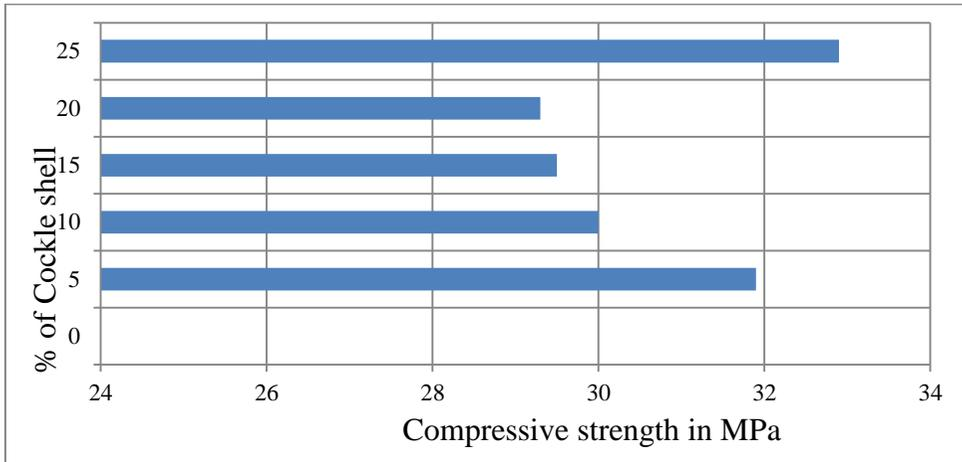
Figure 8 (b): Compressive strength of concrete with different percentage of cockle shell (granite powder 15% fixed)
