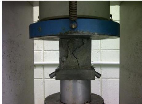
Figure 2: Compression test of mortar cube
