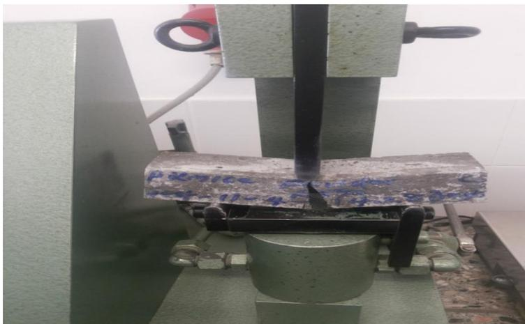
Figure 4: Flexural strength test on pumice ash beam
