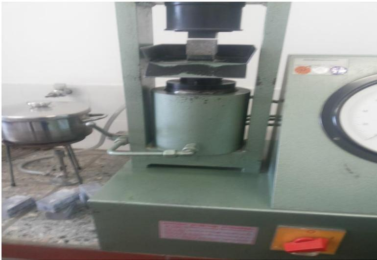
Figure 3: Compressive test on pumice cubes
