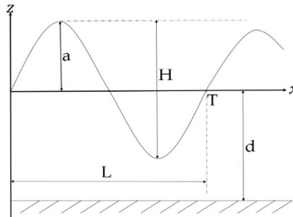
Figure 3: Definition diagram of linear wave theory
