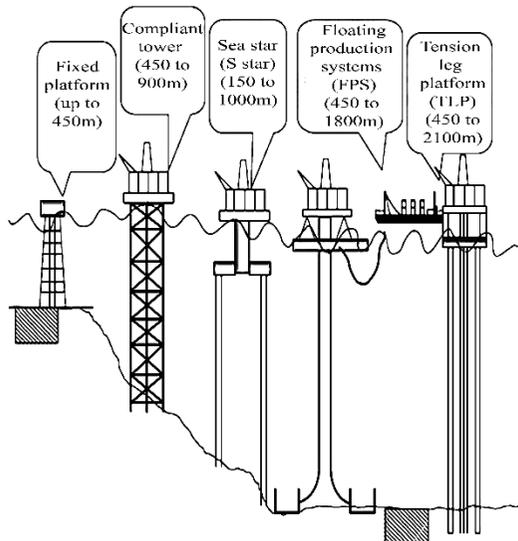
Figure 1: Types of offshore platform (El-Reedy, 2012)
