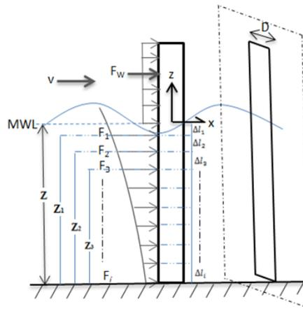
Figure 5: Distribution of forces on structure
