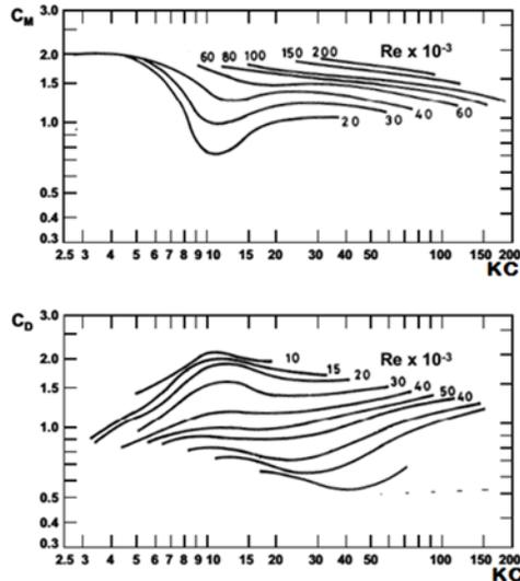
Figure 7: Hydrodynamic coefficient with respect to flow parameter (Chakrabarti 2005)
