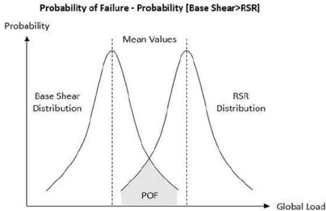
Figure 8: Probability of failure of base shear and RSR distributions
