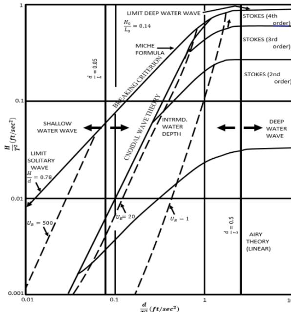
Figure 4: The limits of validity of wave theories (Le Méhauté 1976)
