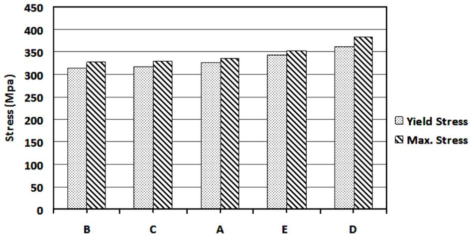
Figure 3: The average results of yield and maximum tensile stress for all groups A, B, C, D and E.
