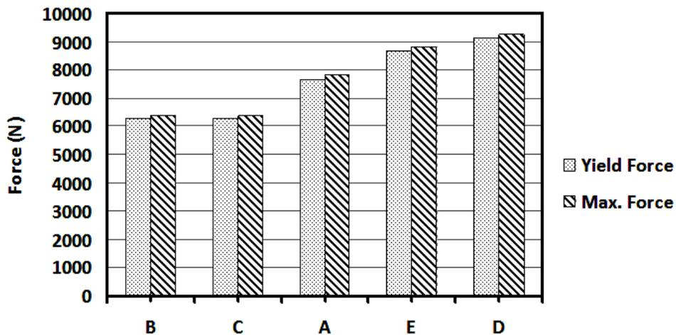
Figure 2: Shows the average results of yield and max. tensile force for all groups A, B, C, D and E.
