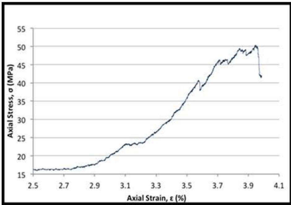
Figure 3: Non-linear Deformation of Kuala Lumpur Limestone
