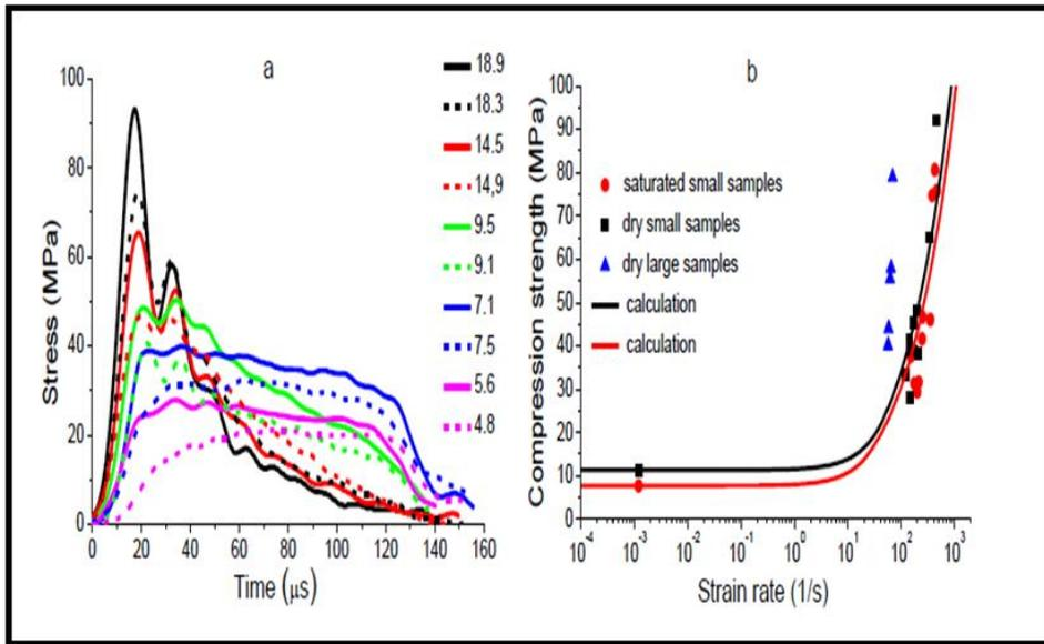
Figure 2: Dynamic stress diagram for different projectile speeds. (dry: bold lines and saturated: dotted lines (a) Classical Kolsky method) and (b) Critical stress in uniaxial compression tests, Dots: experimental data; bold lines: calculated values) (Smirnov *et al.* 2014).
