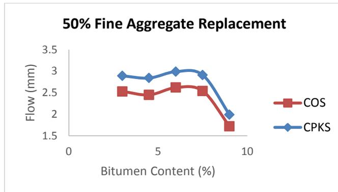
Figure 12: Relationship between Flow and Binder Content at 50% Partial Replacement
