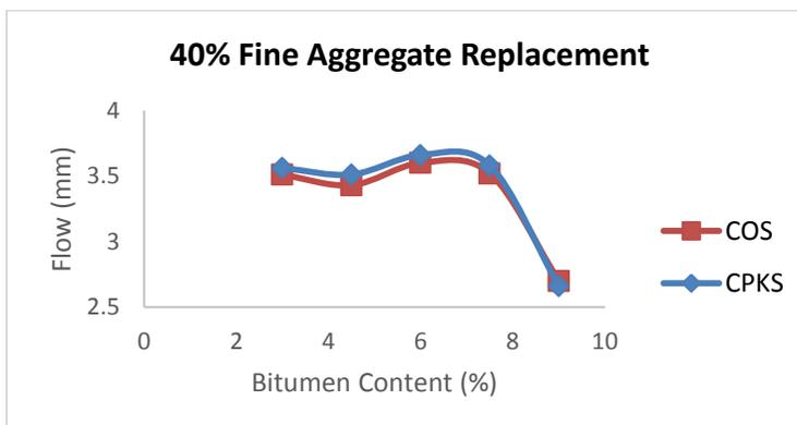
Figure 11: Relationship between Flow and Binder Content at 40% Partial Replacement
