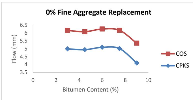
Figure 7: Relationship between Flow and Binder Content at 0% Partial Replacement
