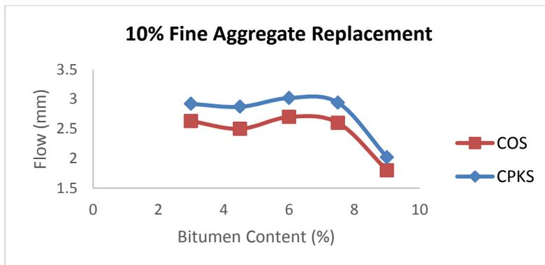
Figure 8: Relationship between Flow and Binder Content at 10% Partial Replacement
