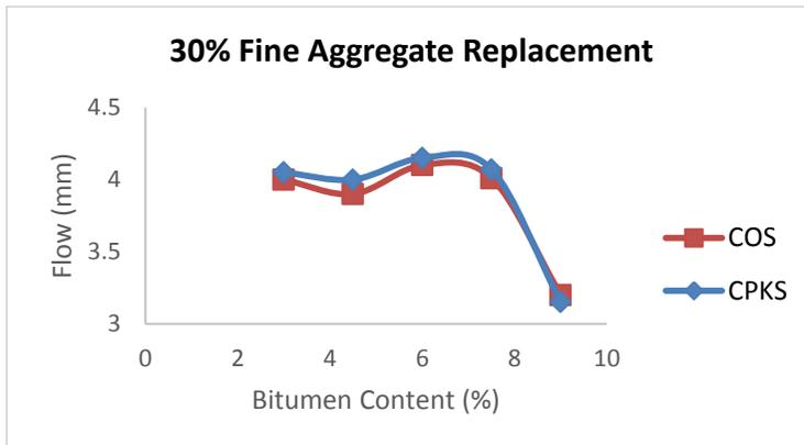
Figure 10: Relationship between Flow and Binder Content at 30% Partial Replacement
