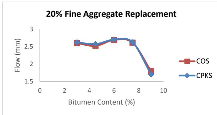
Figure 9: Relationship between Flow and Binder Content at 20% Partial Replacement
