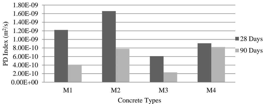
Figure 7: PD index at equal w/c ratio (0.45)
