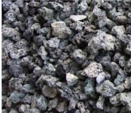
Figure 1: POC used in concrete mix
