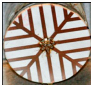
Fig. 6. PCB Star Shield [19]
