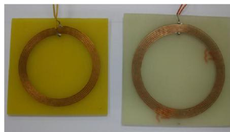
**Fig. 3.** Fabricated circular coil of the transmitter ( $T_x$ ) and receiver ( $R_x$ ) coils
