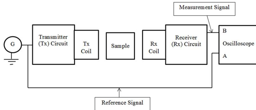
Fig. 4. System Setup Diagram
