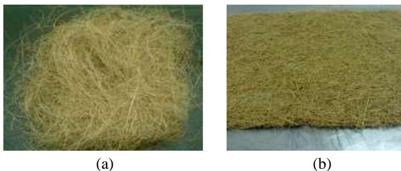
**Fig. 1.** Aspect of the coconut fibers: (a) tangled fibers and (b) pressed mat.
