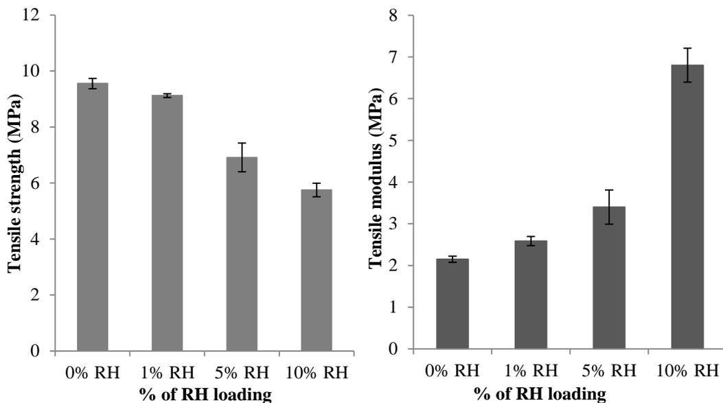
Figure 6. Effects of RH loading on the mechanical properties of ENR/PVC membrane
