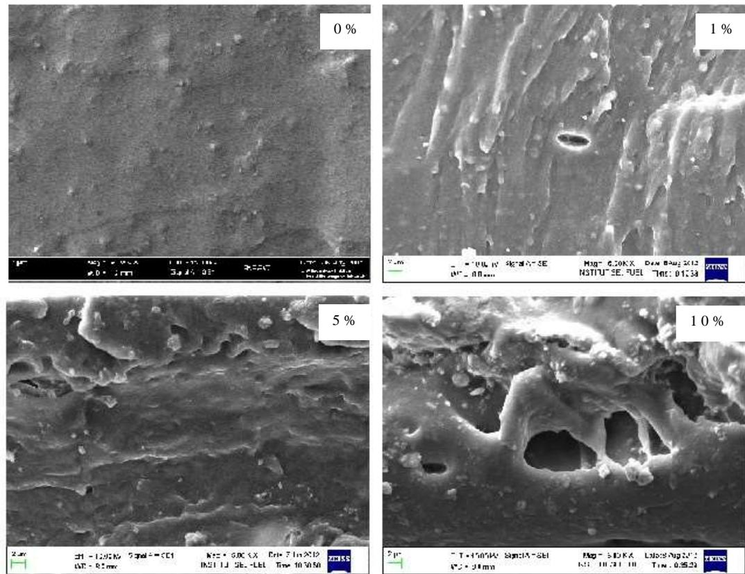
Figure 4. Effects of RH loading on the cross-section of ENR/PVC membrane at magnification of  $\times 5000$
