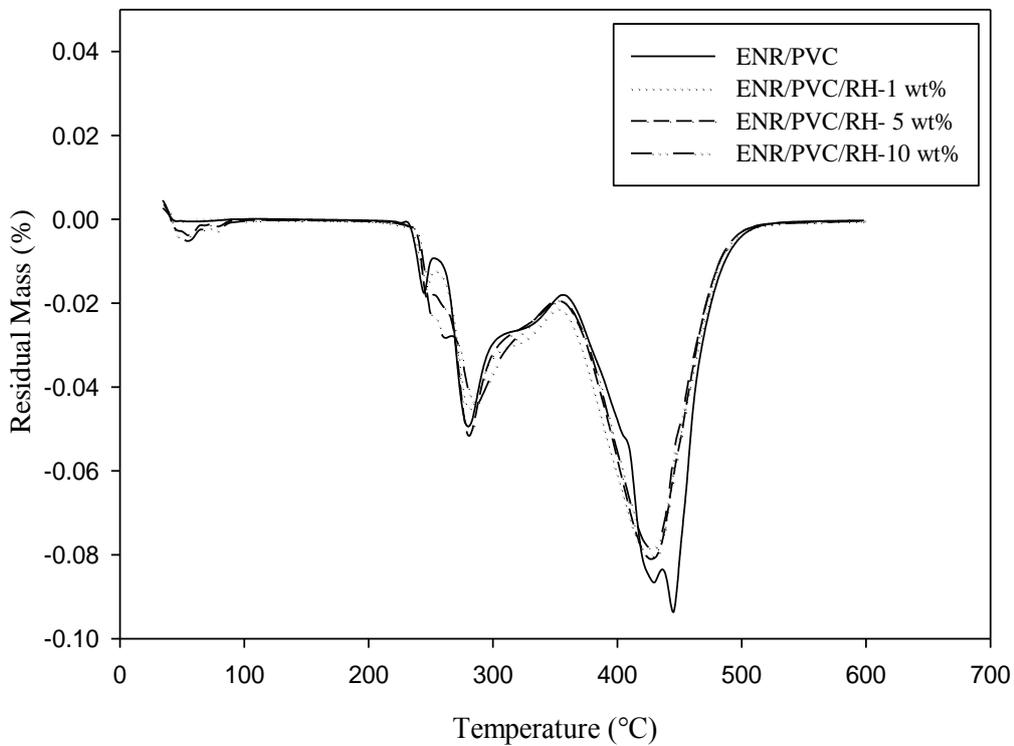
Figure 2. DTG curves for ENR/PVC membrane with various amount of RH
