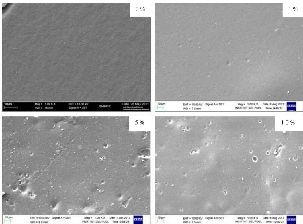
Figure 3. Effects of RH loading on the surface of ENR/PVC membrane at magnification of  $\times 1000$
