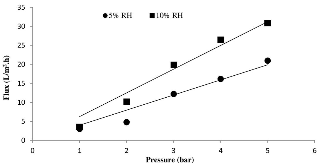
Figure 5. Effects of RH loading on water flux of ENR/PVC membrane
