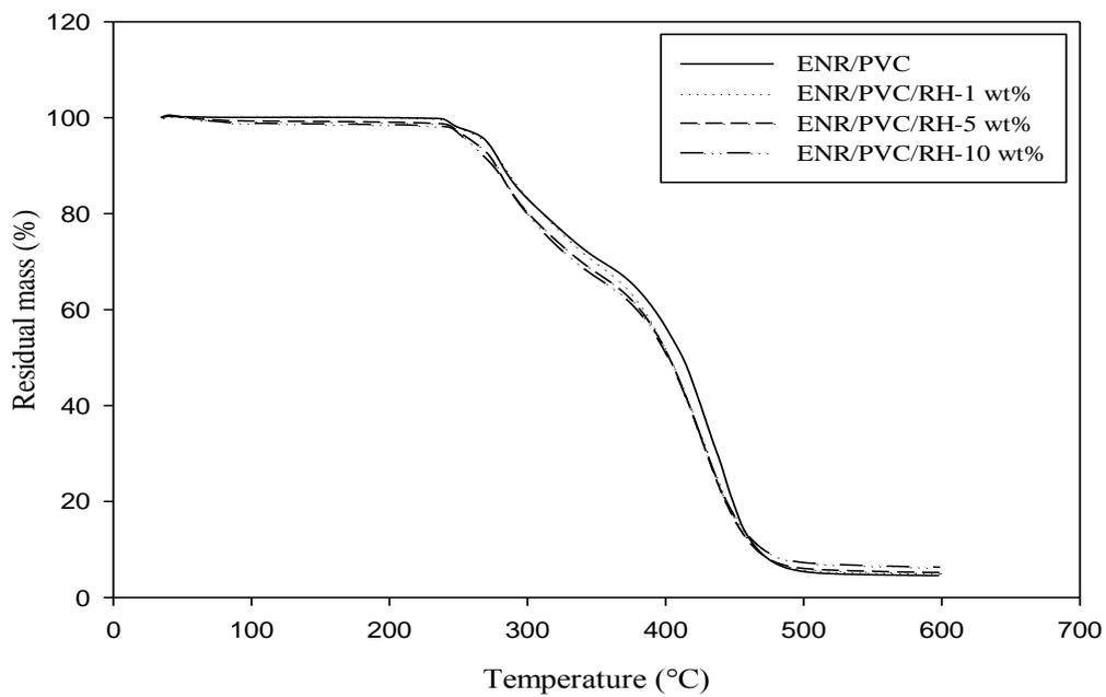
Figure 1. TGA curves for ENR/PVC membrane with various amount of RH
