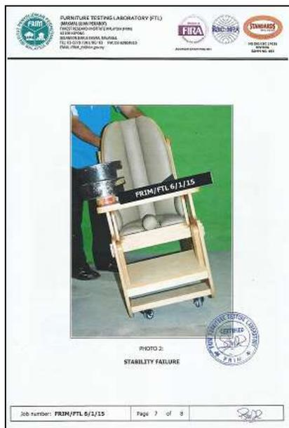
Figure 3: Stability failure
