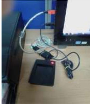
Figure 3: RFID reader connected via USB-RS232 converter to USB port.
