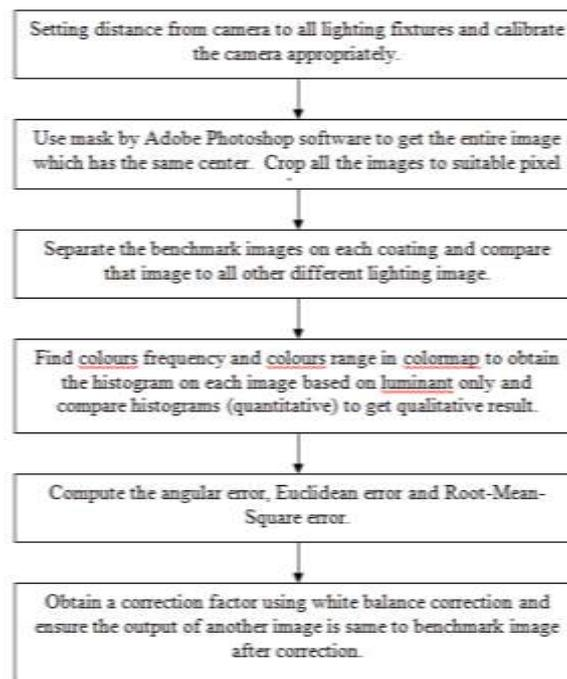
Figure 7: Flow Diagram of the Project method
