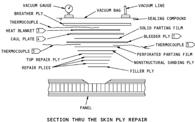
Figure 5. Application of pressure on a skin ply repair.<sup>6</sup>
