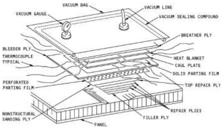
Figure 4. Vacuum bag step sequence for ply replacement.<sup>5</sup>
