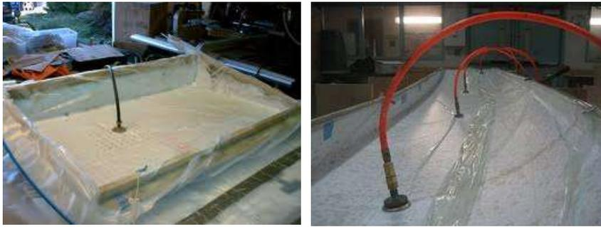
**Figure 2. Hot bonding is accomplished with a heat blanket and used with vacuum bagging<sup>2</sup>**
