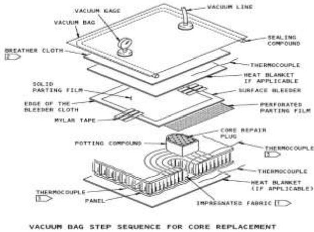
Figure 3. Vacuum bag step sequence for core replacement.<sup>4</sup>
