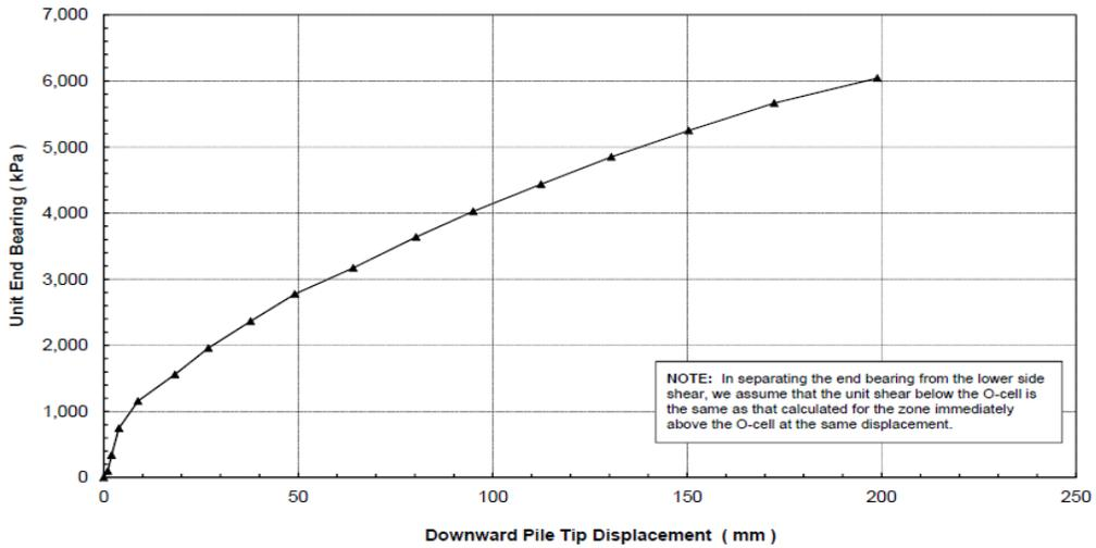
Figure 7: Mobilized Unit Bearing Resistance
