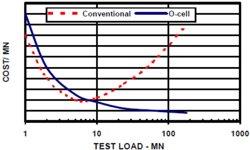
Figure1: Comparison of Load Testing Costs Conventional Vs O-Cell
