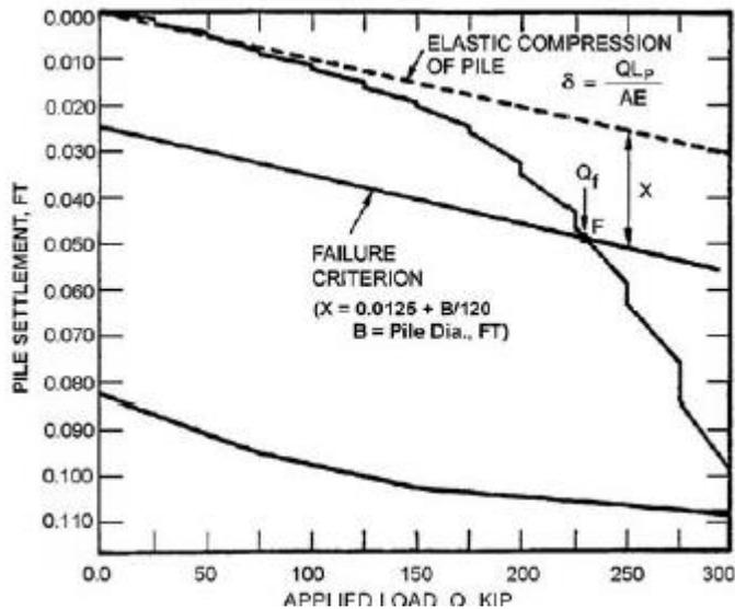
Figure 9: Alternate Method Load Test Interpretation (Modified by Cheney and Chassie, 2000 after Davisson 1972, Source:AASHTO LRFD 2012)
