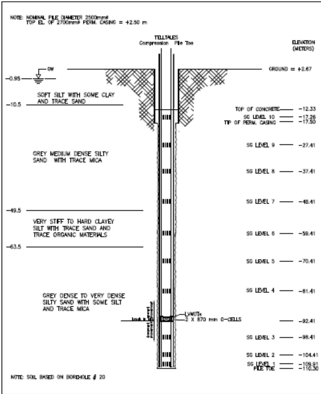
Figure 2: Sub Soil Profile and O-Cell Instrumentation Arrangement
