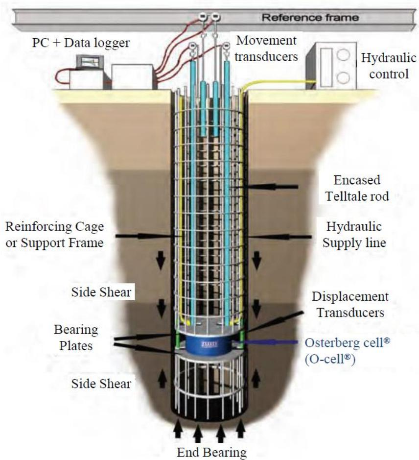
Figure 3: O-Cell Testing Schematic Diagram (Adopted from Loadtest, Inc)
