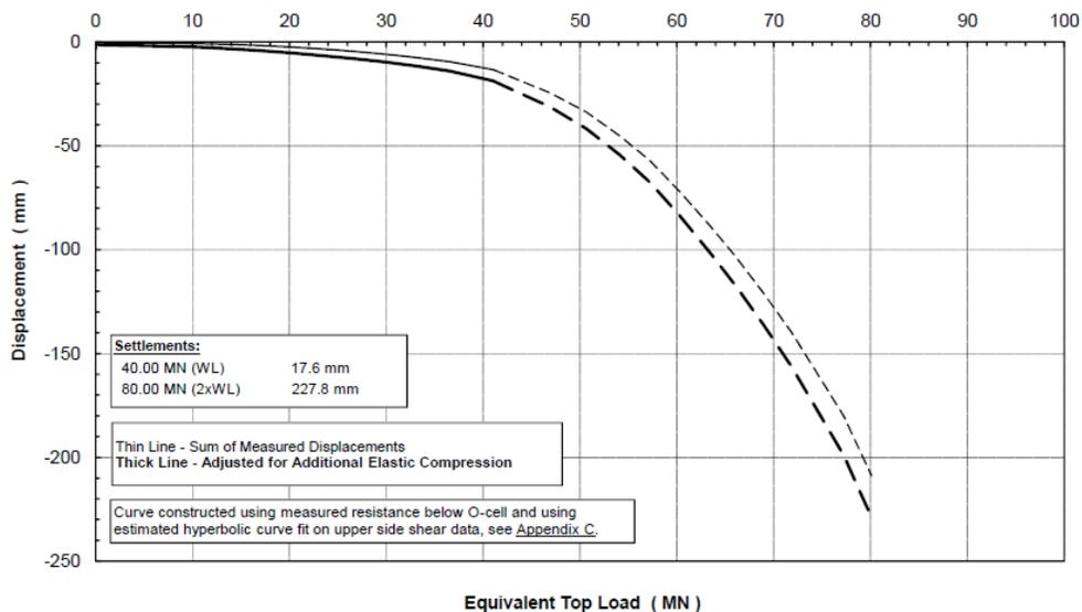
Figure 8: Equivalent Load Settlement Curve
