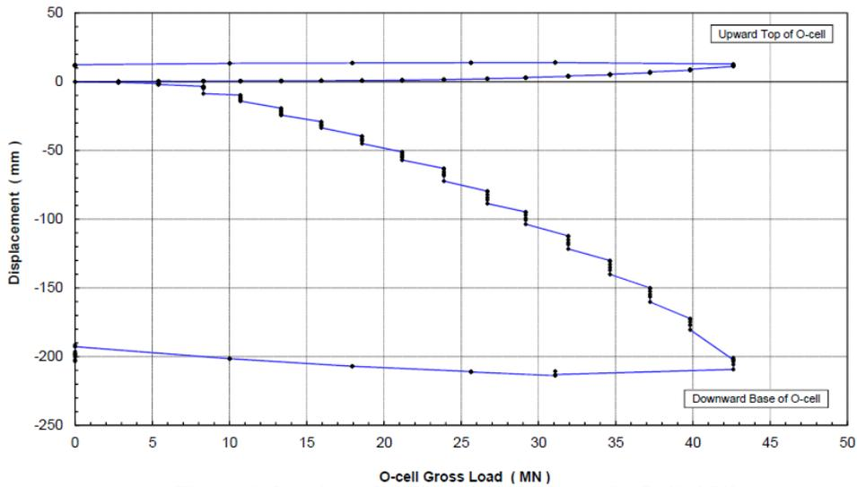
Figure: 5 Osterberg Cell Load-Displacement for Belled Pile
