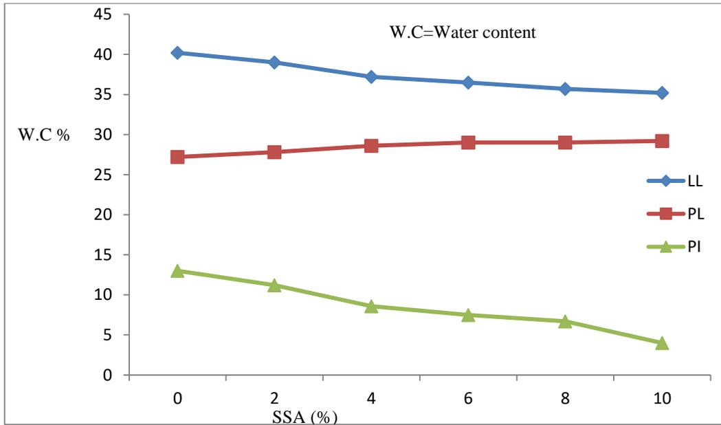
Figure 4. Effects of SSA on atterberg limits of lime-treated lateritic soil
