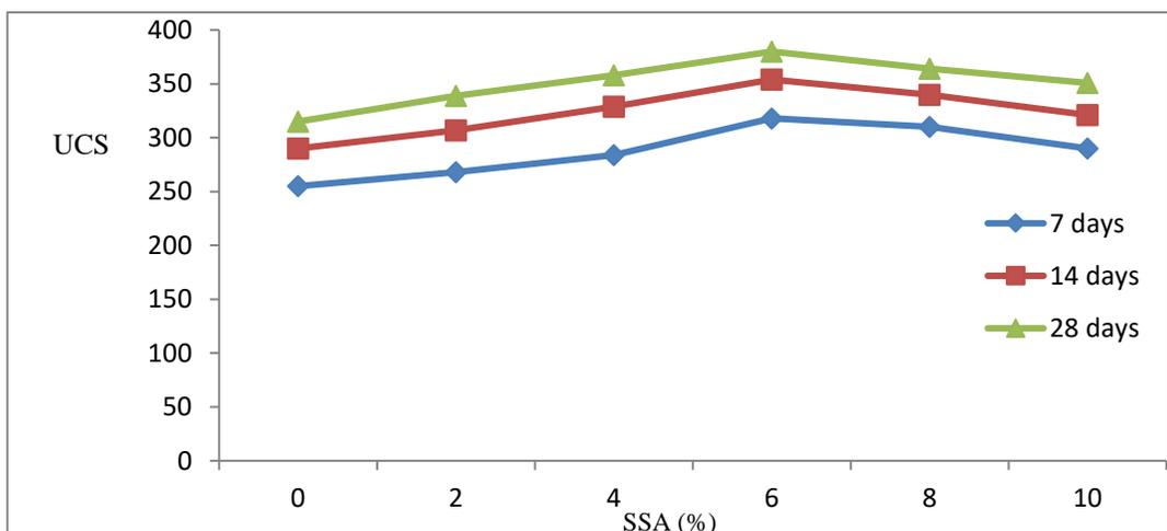
Figure 8. Effect of SSA on UCS of lime-treated lateritic soil
