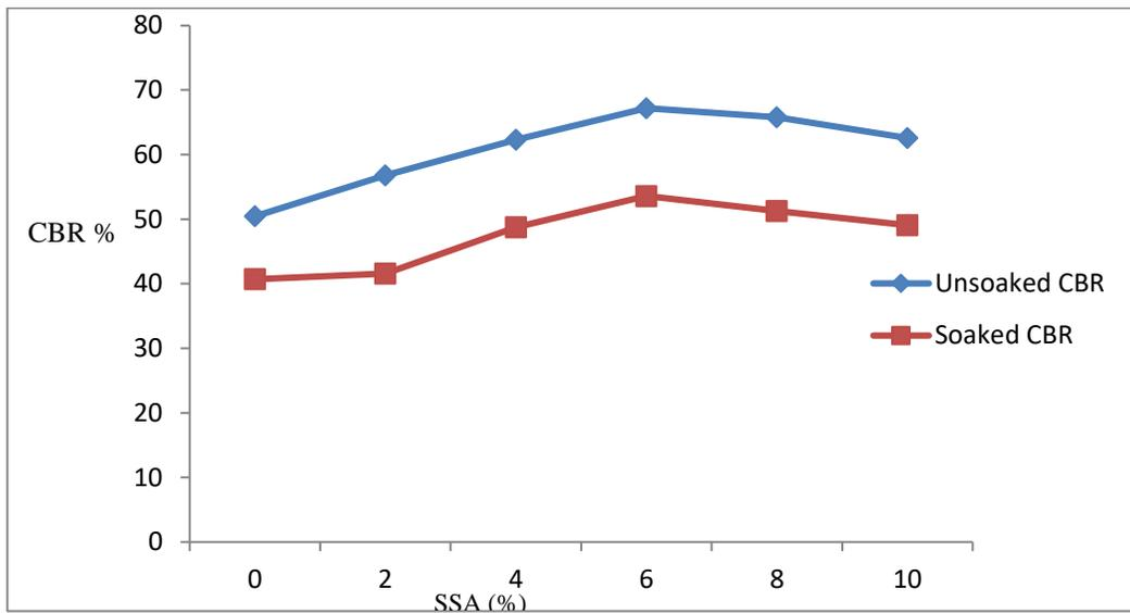
Figure 7. Effects of SSA on CBR of lime-treated lateritic soil
