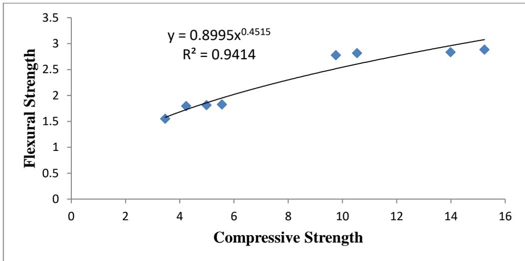
Figure 3: Relationship between Compressive and flexural strength of PKSC
