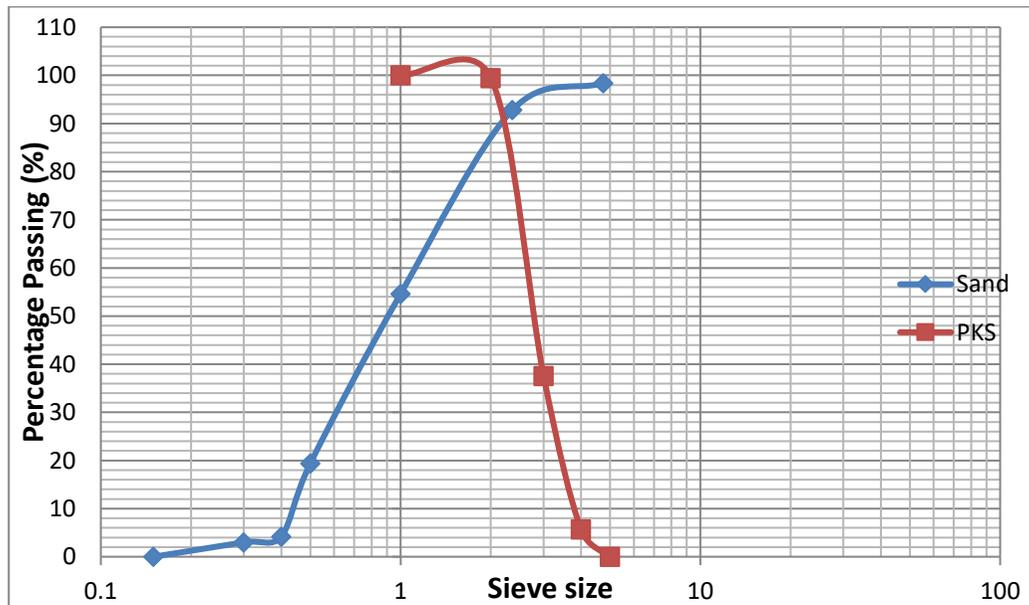
Figure 2: Sieve analysis of Sand and PKS
