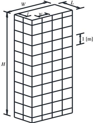
Figure 9: Surface element of the single barrette.
