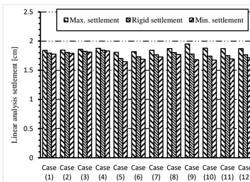
Figure 17: Maximum, minimum and rigid settlement using linear analysis
