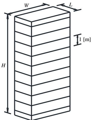
Figure 11: Barrette representing by 1D finite elements.
