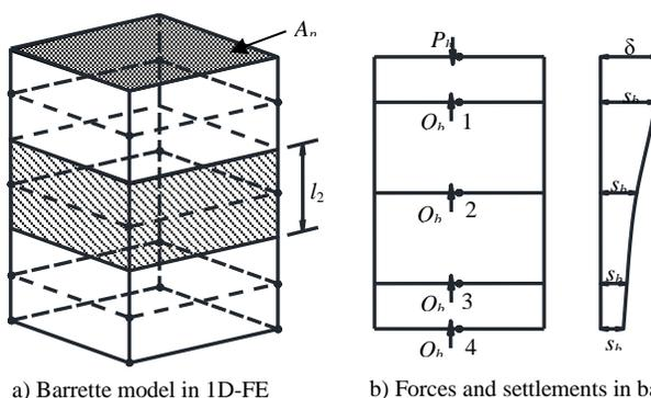
Figure 4: Finite element mesh of barrette and element geometry
