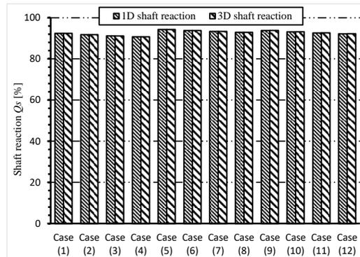
Figure 14: Shaft reaction using 1D and 3D finite elements.
