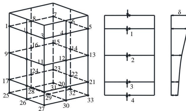
Figure 3: Surface mesh of the barrette with node numbering, loads and settlement
