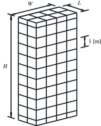
Figure 10: Barrette representing by 3D finite elements.
