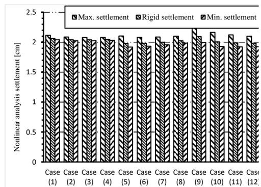
Figure 18: Maximum, minimum and rigid settlement using nonlinear analysis
