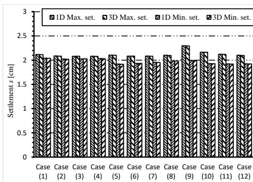
Figure 15: Max. and Min. settlement when using 1D and 3D finite elements.
