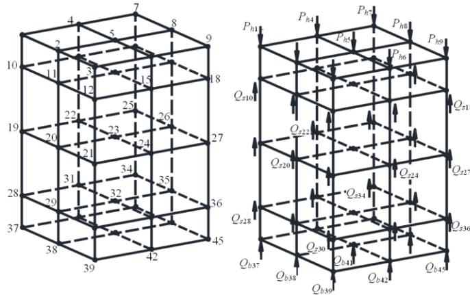
Figure 2: Mesh of the barrette with node numbering, loads and settlement
