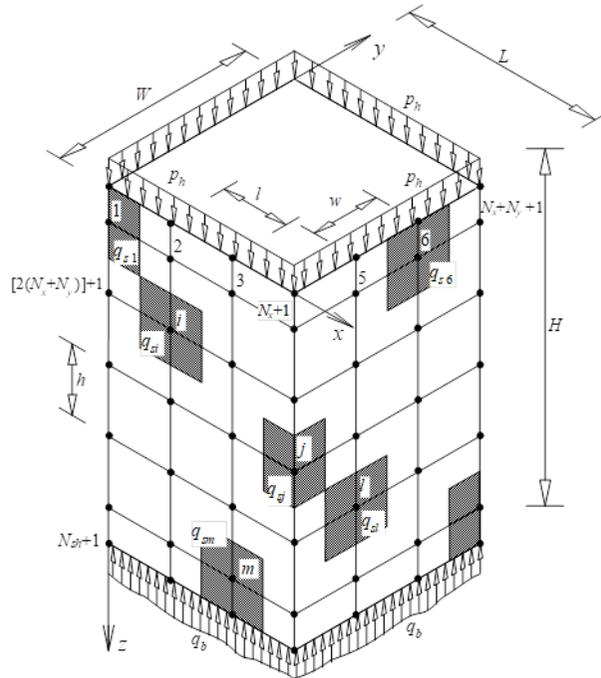
Figure 1: Barrette geometry, elements and stresses
