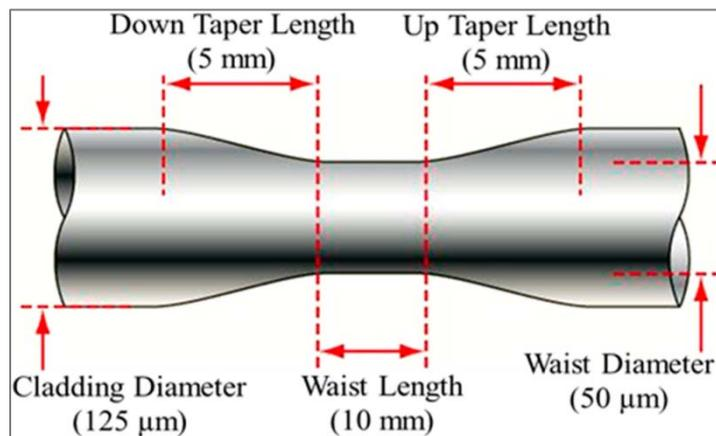
Figure 1: Tapered optical fiber parameters (Shabaneh, et al., 2014)
