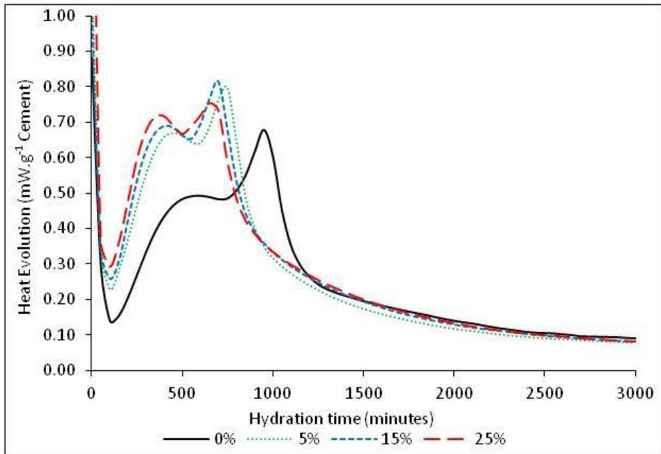
Figure 1: Isothermal profile for the hydration of mortar containing synthetic drill cuttings
